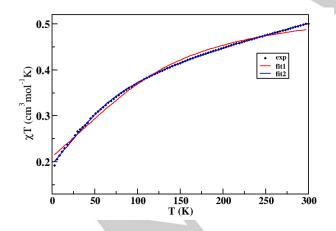
**Figure 2:** Molar magnetic susceptibility as a function of temperature with a field of 1 T for the  $Li_2Np^{VI}O_2(DPA)_2 \cdot 2H_2O$  compound. The red and blue lines show the fits using Eq. 21 without and with TIP respectively.
