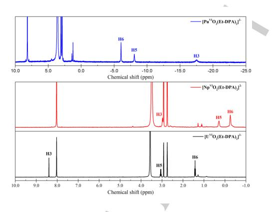
Figure 3: <sup>1</sup>H NMR spectra of  $[An^{VI}O_2(Et - DPA)_2]^{2-}$  complexes at 298 K in  $[D_7]DMF$  at 9.4 T.
