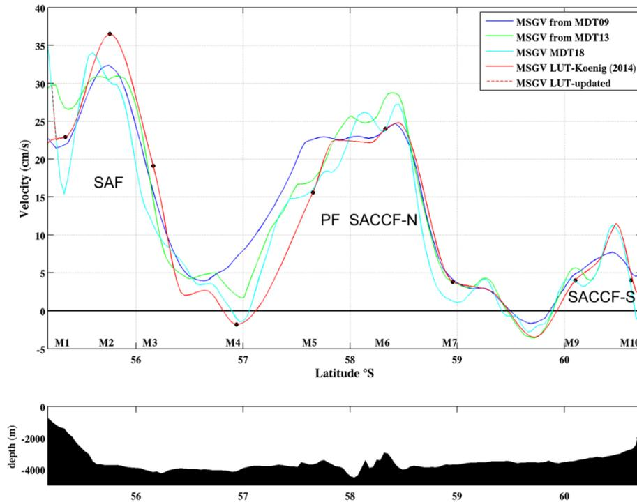
**Figure 19.** Mean surface geostrophic velocities (MSGVs) derived from MDT CNES-CLS09 (blue), from MDT CNES-CLS13 (green), MDT CNES-CLS18 (cyan) and LUT (red) along Jason track no. 104. Location of the Drake moorings are indicated M1 to M10. Below bathymetry along the section.
