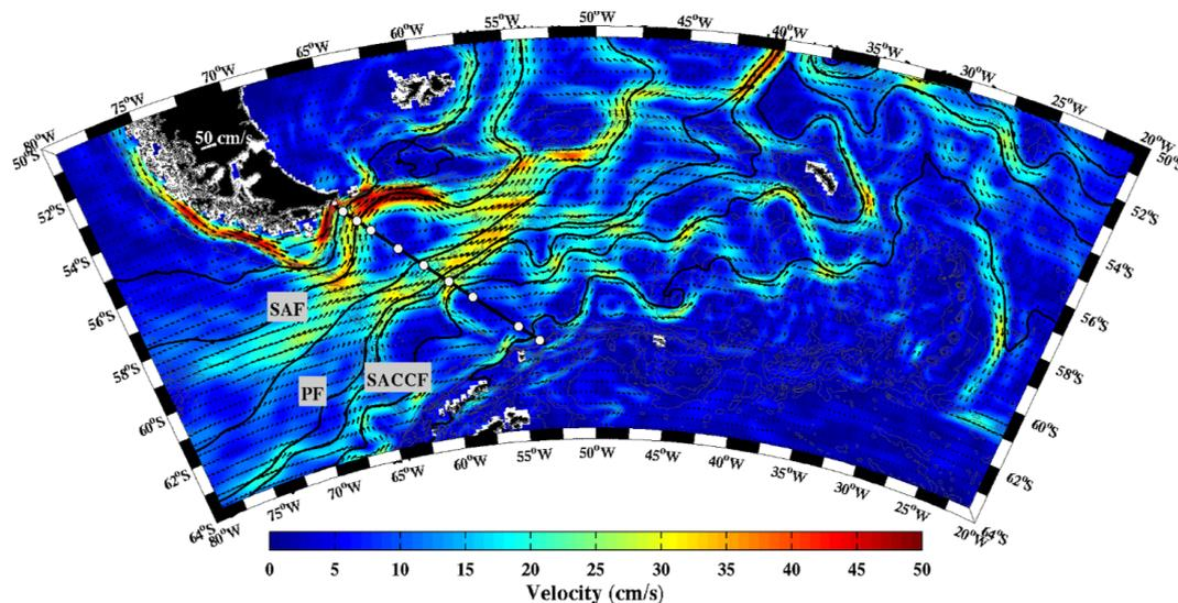
**Figure 18.** Mean surface velocity magnitude (in  $\text{cm s}^{-1}$ ) and mean surface velocity vectors from MDT CNES-CLS18. Black lines are isolines of mean sea surface height corresponding to the main Antarctic Circumpolar Current (ACC) fronts and their branches: SAF-N (23 cm), SAF-M (0 cm), PF-N (43 cm), PF-M ( $-70$  cm), PF-S ( $-79$  cm), SACCF-N ( $-93$  cm) and SACCF-S ( $-114$  cm). White dots indicate the position of the DRAKE moorings.
