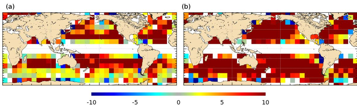
**Figure 2.** Difference ( $\text{cm s}^{-1}$ ) of the RMSD obtained using the first guess of MDT CNES-CLS13 and the first guess of MDT CNES-CLS18 for the (a) zonal and (b) meridional components in  $5^\circ \times 5^\circ$  boxes. Only boxes with more than 500 points and where difference is statistically significant at more than 95 % ( $T$  test) are shown. The reddish colors denote improvement while bluish colors stand for degradation (see text for more details).
