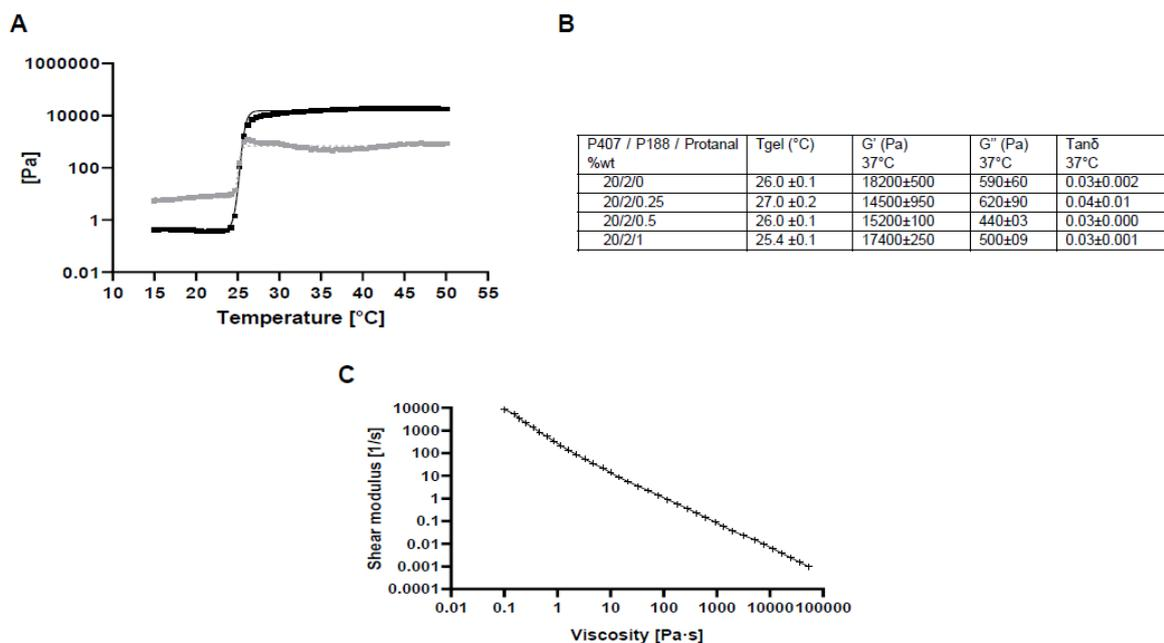
Figure 1 : P407/P188/alginate thermogel rheological results. (A) Representation of the sigmoidal fitting curve of the viscous modulus  $G''$  (grey) and the elastic modulus  $G'$  (black) for 20/2/1 thermogel. (B) Rheological parameters of the different formulations tested.  $n=3$  mean  $\pm$ SD. (C) Spearman correlation between shear modulus and viscosity for the P407/P188/alginate 20/2/1 formulation ( $n=6$ ,  $P<0,0001$ \*\*\*\*).
