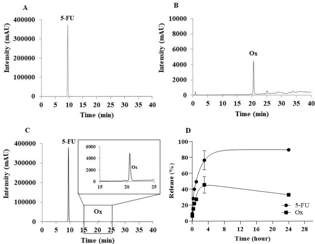
Figure 4: HPLC chromatograms of (A) 5-FU WFI, (B) Ox WFI and (C) 5-FU/Ox admixture at 266 nm (maximal wavelength of 5-FU). (D) determination of 5-FU and Ox concentrations in 5-FU/Ox admixture, prepared in WFI or thermogel, over time at 4°C (n=3).
