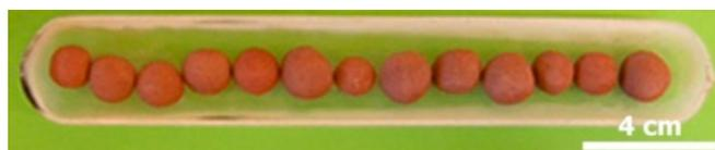
Figure 1. Optical image of the (hematite + W-PVC + clay) pellets mixtures.
