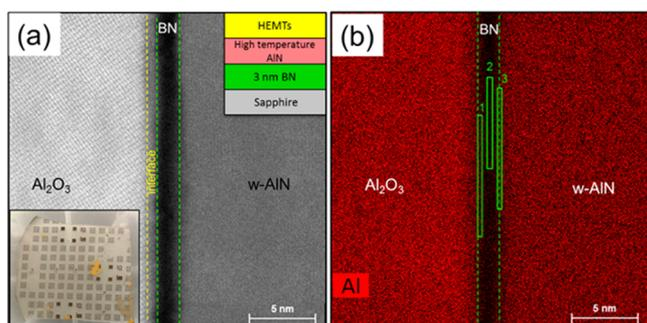
**Figure 5.** Cross-sectional bright-field HAADF-STEM image (a) and energy-dispersive X-ray spectroscopy (EDX) elemental mappings of Al (b) of HEMTs/high-temperature AlN/3 nm h-BN grown on sapphire. Inset in (a): schematic illustration of the grown structure photograph of the device after attempted lift-off.
