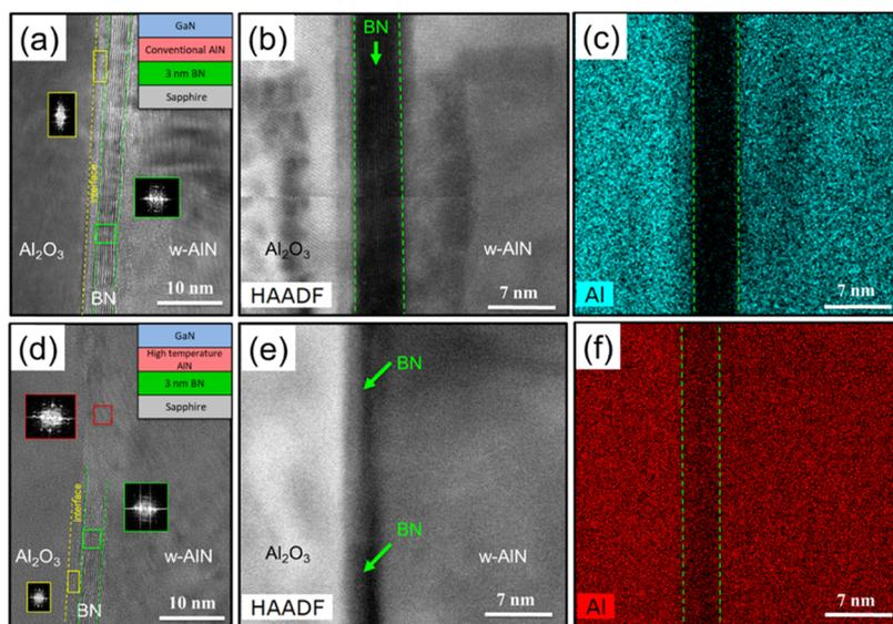
**Figure 2.** Cross-sectional high-resolution TEM and bright-field HAADF-STEM images, and energy-dispersive X-ray spectroscopy (EDX) elemental mappings of Al of GaN/conventional AlN/h-BN (a–c) and GaN/high-temperature AlN/h-BN (d–f) grown on sapphire, respectively. Insets of (a) and (d): schematic illustration of the grown structure.
