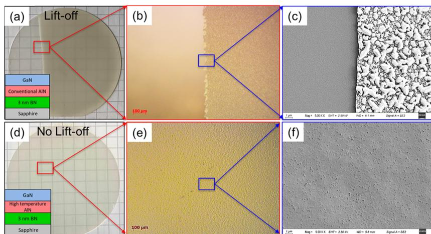
**Figure 1.** Photograph, optical microscope, and SEM images of GaN/conventional AlN/h-BN (a–c) and GaN/high-temperature AlN/h-BN (d–f) grown on sapphire, respectively. Insets of (a) and (d): schematic illustration of the grown structures.
