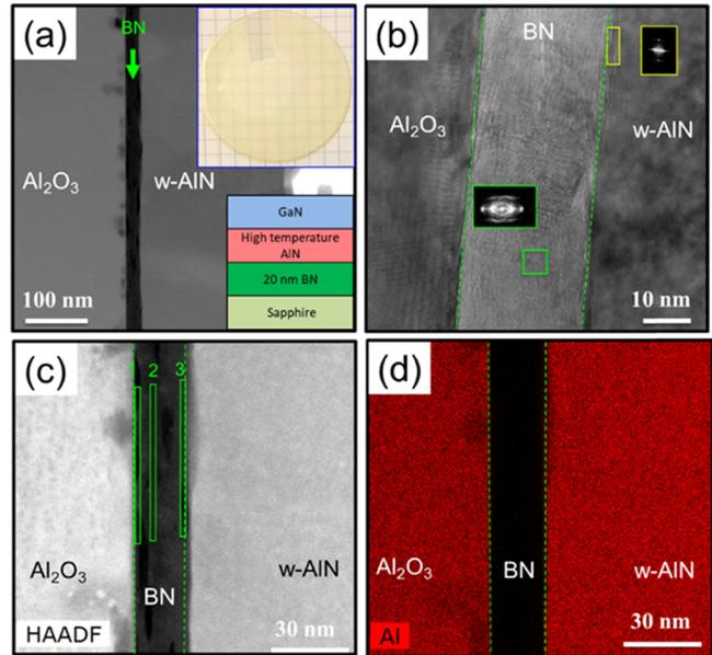
**Figure 4.** Cross-sectional high-resolution TEM and bright-field HAADF-STEM images, and the energy-dispersive X-ray spectroscopy (EDX) elemental mappings of Al of GaN/high-temperature AlN on 25 nm h-BN grown on sapphire, respectively. Inset: schematic illustration of the grown structure and the photograph of the sample after lift-off.
