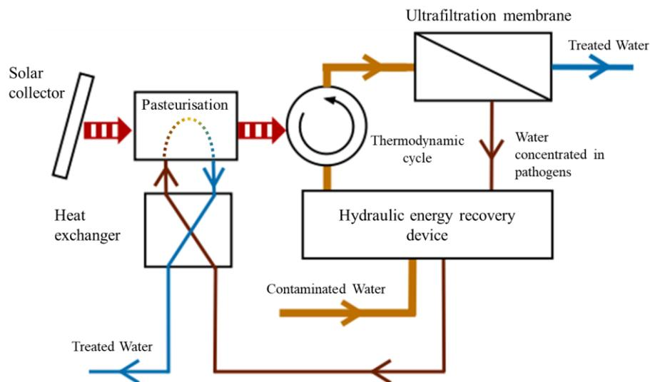
Fig. 3. Block diagram of the hybrid process
