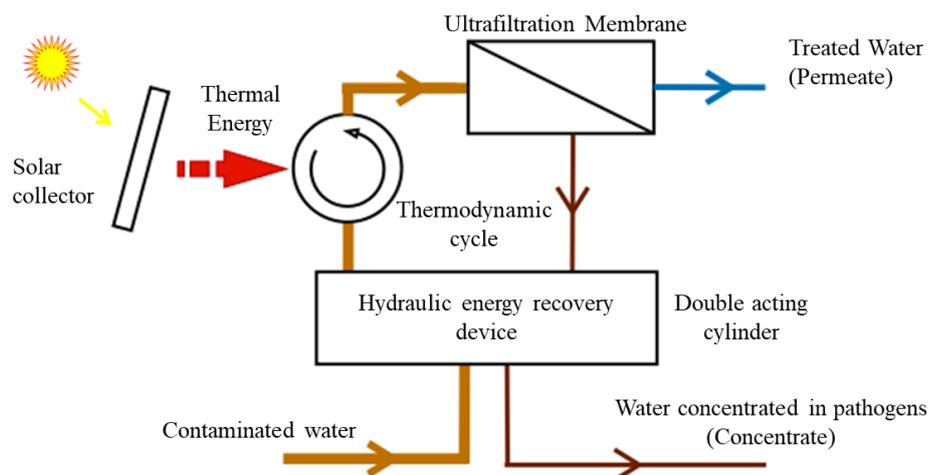
*Fig. 1. Block diagram of the membrane filtration process*
