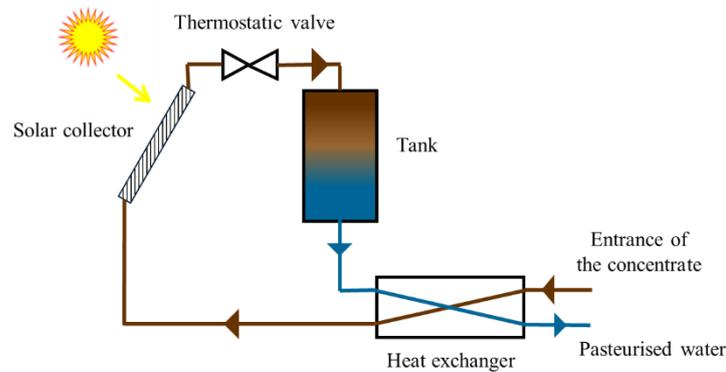
Fig. 2. Diagram of the pasteurisation process
