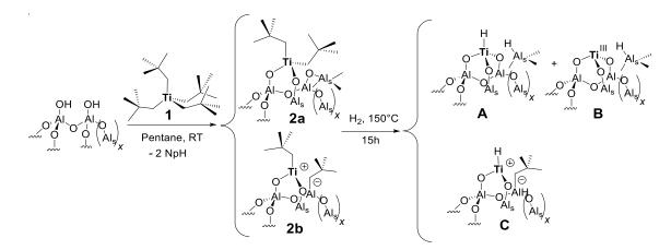
Scheme 1. Grafting reaction of TiNp<sub>4</sub>, 1, onto  $Al_2O_{3-500}$  leading to neutral, 2a, and cationic, 2b, surface species and preparation of alumina supported titanium hydrides, [Ti-H]@Al<sub>2</sub>O<sub>3-500</sub>, leading to neutral Ti(IV) hydride, A, Ti(III), B, and Ti(IV) cationic hydride, C.
