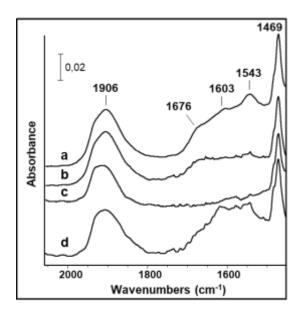
**Figure 2.** *In situ* FTIR spectra obtained after subtraction of the alumina support contribution: a)  $[Ti-H]@Al_2O_{3-500}$ ; b)  $[Ti-H]@Al_2O_{3-500}$  treated under D<sub>2</sub> for 1h at 25 °C; c) **b** under D<sub>2</sub> overnight; d) reaction of **c** with H<sub>2</sub> for 1h at 150°C.
