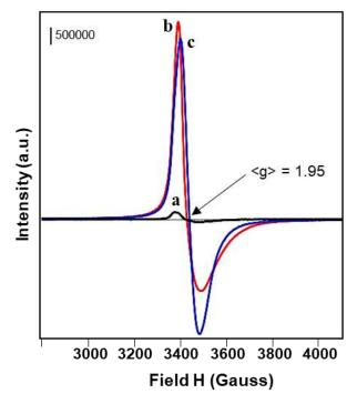
**Figure 4:** ESR patterns of paramagnetic species on the surface of Al<sub>2</sub>O<sub>3-500</sub>: a TiNp<sub>x</sub>@Al<sub>2</sub>O<sub>3-500</sub> (black); b- [Ti-H]@Al<sub>2</sub>O<sub>3-500</sub> (red); c- after the butanolysis of [Ti-H]@Al<sub>2</sub>O<sub>3-500</sub> (blue).
