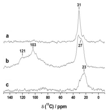
**Figure 3.** <sup>13</sup>C CP-MAS solid-state NMR spectra of **a.**  $TiNp_x@Al_2O_{3-500}$ ; **b.** <sup>13</sup>C enriched  $TiNp_x@Al_2O_{3-500}$  and **c.**  $[Ti-H]@Al_2O_{3-500}$  obtained from the hydrogenolysis of <sup>13</sup>C enriched  $TiNp_x@Al_2O_{3-500}$ .
