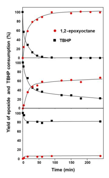
**Figure 5:** Activity of supported [Ti-H] species for 1-octene epoxidation by TBHP: yield of 1,2-epoxyoctane and conversion of TBHP a) [Ti-H]@SiO<sub>2-500</sub>; b) [Ti-H]@SiO<sub>2</sub>-Al<sub>2</sub>O<sub>3-500</sub>; c) [[Ti-H]@Al<sub>2</sub>O<sub>3-500</sub>.
