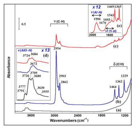
**Figure 1.** *In situ* FTIR spectra of a) Al<sub>2</sub>O<sub>3-500</sub>, activated at 500 °C under vacuum overnight; b) after grafting of TiNp<sub>4</sub> on Al<sub>2</sub>O<sub>3-500</sub>; c) after treatment of the resulted supported species by hydrogen for 12 h at 150 °C; d) Enlargement showing the evolution of the  $v_{(AIO-H)}$  area; e) Enlargement of the  $v_{(AI-H)}$  and  $v_{(Ti-H)}$  area, obtained after subtraction of a) to c).
