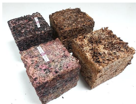
Figure 3: Cubic samples for thermal and compression test
