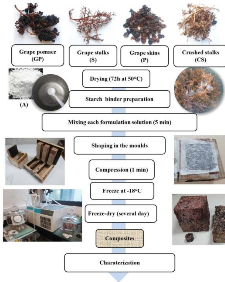
Figure 2: Synthetic diagram of the step of composite manufacturing
