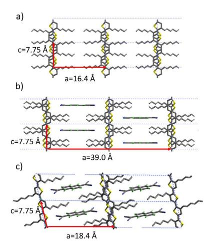
**Figure 6**. b-axis projections of the structural models of a) P3HT (form I), ii) the trial structure of P3HT- $F_6$ TCNNQ and c) the final refined structure after energy minimization. Hydrogen atoms are omitted for clarity.
