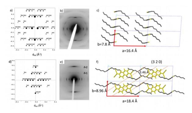
**Figure 5**. Calculated (a and d) and experimental (b and e) electron diffraction patterns for the  $[0\ 1\ 0]$  zone for P3HT (form I) (a and b) and P3HT-F<sub>6</sub>TCNNQ (d and e). The form I structure is taken from reference [30] whereas the doped P3HT structure is refined and corresponds to the model illustrated in Figure 6. In c) and f), the c-axis projection of the pristine and doped structures are shown, respectively.
