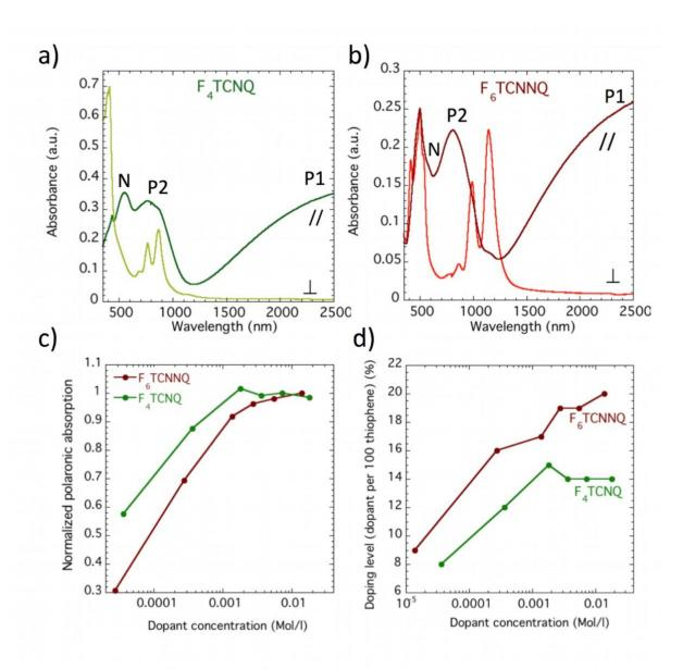
Figure 2. Polarized UV-vis-NIR spectra of oriented P3HT films featuring highly polarized polaronic absorption bands (P1, P2) for incident light polarized parallel to the rubbing direction (II) and the polarized absorption bands of the anion for incident light polarized
