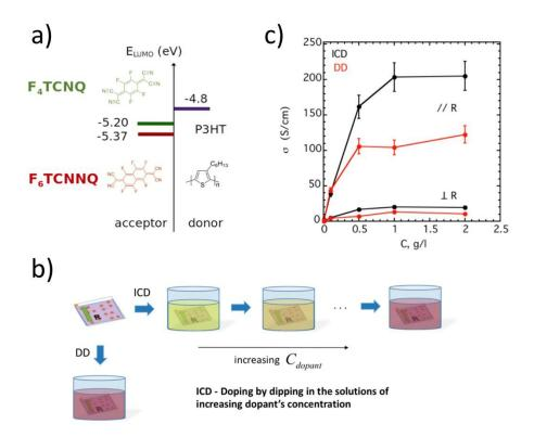
**Figure 1.** a) Energy diagram of the LUMO levels of F<sub>4</sub>TCNQ, F<sub>6</sub>TCNNQ and HOMO of P3HT, b) Schematic illustration of incremental concentration doping (ICD) and direct doping (DD) methods, c) Comparison of the electrical conductivity of oriented P3HT films doped with F<sub>4</sub>TCNQ in acetonitrile by the two doping methods as a function of increasing dopant concentration.
