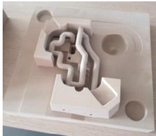
Figure 3: Design of conformal heating channels (left), and 3D printed sand half mold (right).
