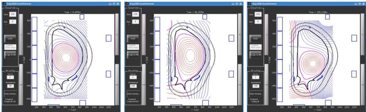
Figure 2: Examples of plasma equilibria at times 5.9s, 66.3s and 133.1s from the IDS database populated from a 280s DINA simulation of ITER
