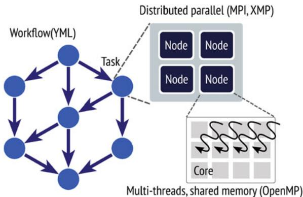
Fig. 1 An overview of multi-SPMD programming model
