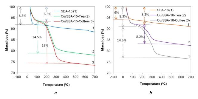
Fig. 8 TGA patterns of SBA-15 and Cu/SBA-15 (a) and SBA-16 and Cu/SBA-16 (b).
