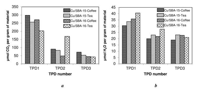
Fig. 13 Repetitive CO<sub>2</sub>-TPD (a) and H<sub>2</sub>O-TPD (b) profiles for Cu/SBA samples. These values were accurately assessed by the area of the TPD patterns between 20 °C and 150 °C. This temperature range is based on the thermal stability threshold established at 170 °C
