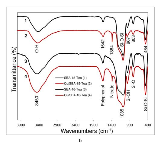
Fig. 9 FTIR diagrams of: Coffee- (a) and Tea-treated SBA samples (b)
