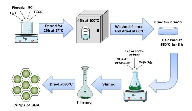
Scheme. 1 Illustration of the different steps of the protocol for the synthesis of SBA-supported copper nanoparticles and characterization
