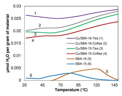
**Fig. 11** TPD patterns of water for SBA and CuNP-SBA samples. These purely qualitative TPD were achieved after dynamic impregnation with CO<sub>2</sub> at 20 °C under a 15 mL.min<sup>-1</sup> dry nitrogen stream, followed by a purge at room temperature and TPD up to 150 °C (200 mL CO<sub>2</sub> for 45–50 mg dry adsorbent). These first TPD runs cannot be repeated for the same materials, given that the decomposition of organic dispersing agents triggers at ca. 170 °C
