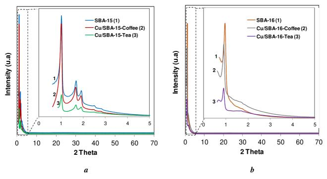
**Fig. 1** Small and large angle XRD patterns for SBA-15 and Cu/SBA-15 (**a**) and SBA-16 and Cu/SBA-16 (**b**).
