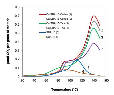
**Fig. 10** TPD patterns of CO<sub>2</sub> for SBA and CuNP-SBA samples. These purely qualitative TPD were achieved after dynamic impregnation with CO<sub>2</sub> at 20 °C under a 15 mL.min<sup>-1</sup> dry nitrogen stream, followed by a purge at room temperature and TPD up to 150 °C (200 mL CO<sub>2</sub> for 45–50 mg dry adsorbent). These first TPD runs cannot be repeated for the same materials, given that the decomposition of organic dispersing agents triggers at ca. 170 °C
