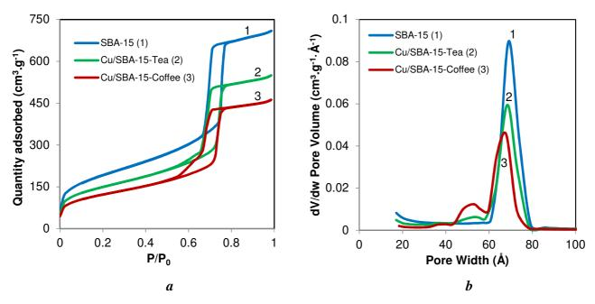
**Fig. 2** N<sub>2</sub> adsorption/desorption isotherms (**a**) and pore size distribution (**b**) of SBA-15 and its modified counterparts
