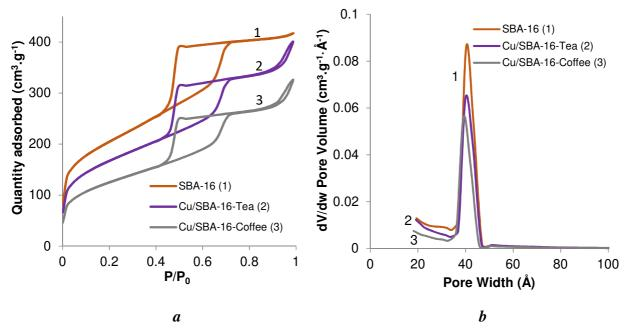
**Fig. 3** N<sub>2</sub> adsorption/desorption isotherms (**a**) and pore size distribution (**b**) of SBA-16 and its modified counterparts
