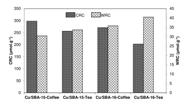
**Fig. 12** CRC versus WRC of Cu/SBA materials. These values were accurately assessed by the area of the TPD patterns between 20 °C and 150 °C. This temperature range is based on the thermal stability threshold established at 170 °C
