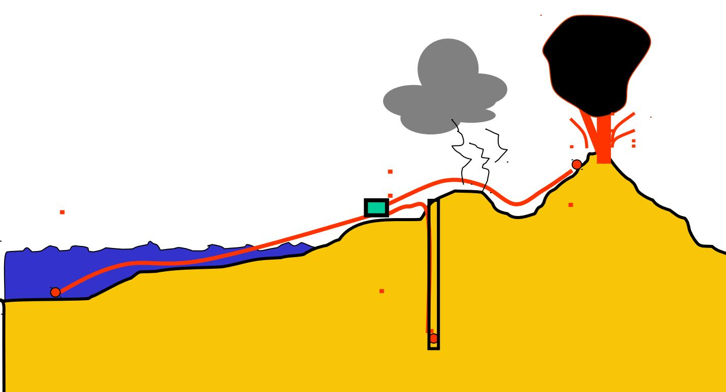
In many areas with high telluric hazard, our understanding of the seismogenic and mechanical processes is limited by the difficulty or impossibility to deploy arrays of high performance seismometers or of other geophysical sensors, due to high cost (e.g. offshore) and/or hazard (e.g., lightning, active volcano, high T in boreholes...) of the maintenance.
