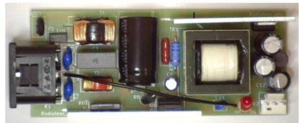
Fig. 9. Picture of the designed and tested SMPS.
