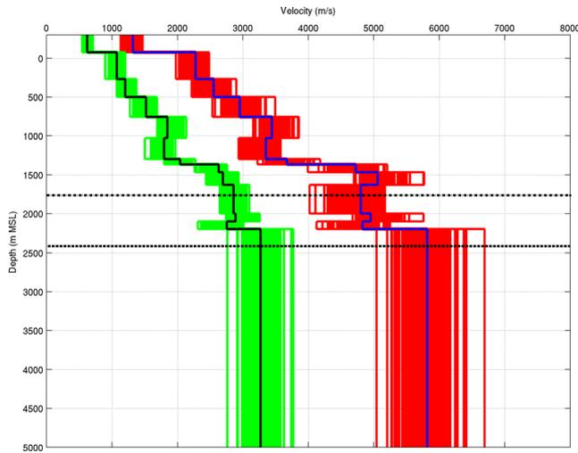
**Figure 5.** Profiles of the reference  $P$ -wave (blue curve) and  $S$ -wave (black curve) velocities at Rittershoffen overlaying the 150 random profiles for the  $P$ -wave (red curves) and the  $S$ -wave (green curve) velocities (see Section 4.2.1 for details). The bottom depth of the well GRT1 (horizontal dashed line) and the upper depth of the injection zone (horizontal dotted-dashed line) are also shown.
