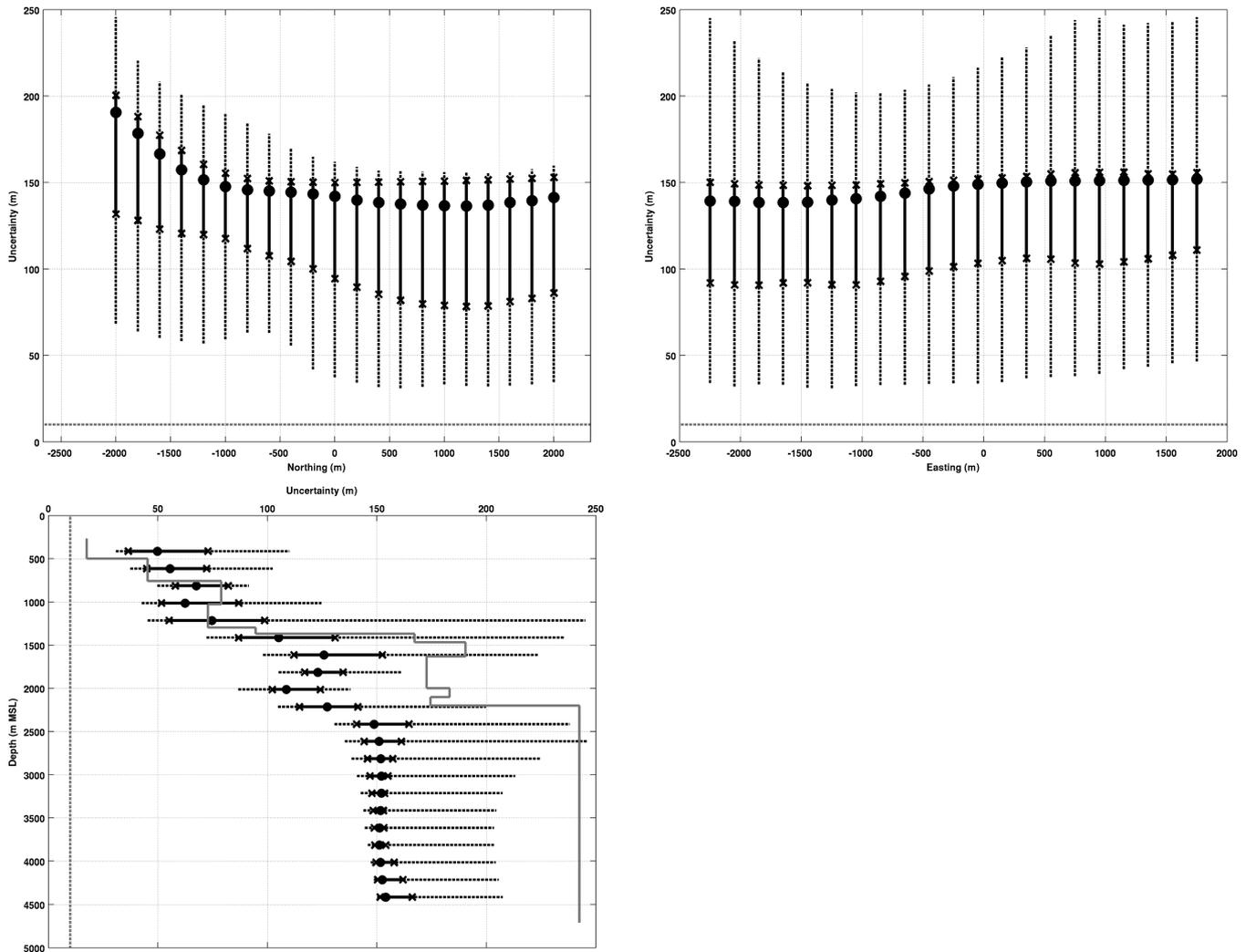
**Figure 8.** Boxplots of the location uncertainties as a function of latitude (top left), longitude (top right) and depth (bottom left). The uncertainties median (points), 25th and 75th percentiles (crosses), and range (dotted segment) are shown. The 10-m relocation-mesh size is displayed (grey dashed-line) as reference.
