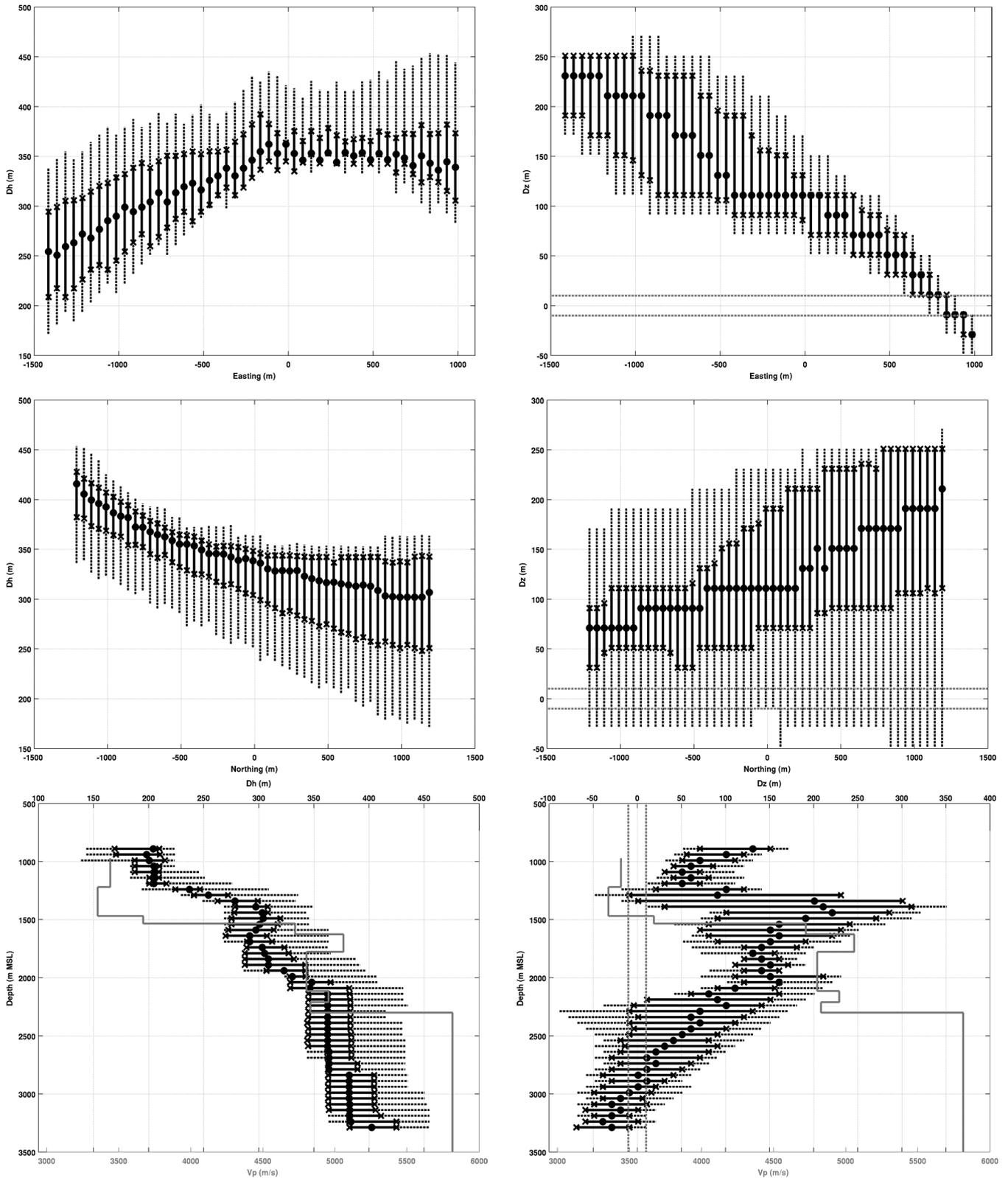
**Figure 15.** Boxplots of the horizontal (left column) and vertical (right column) inaccuracies for the horizontal plane along east (top row) and along north (middle row) and for the N–S vertical plane along depth (bottom row). For details on the symbols, see Fig. 8.
