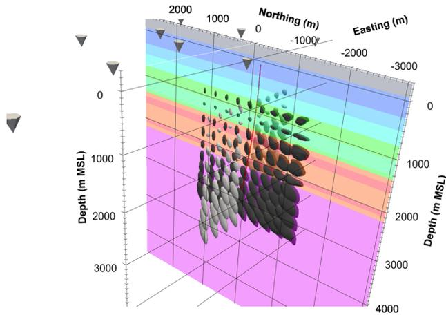
**Figure 10.** 3-D view of the relocation uncertainties at 68.3 per cent confidence levels for the 81 sources distributed every 300 m in the E–W vertical plane (light grey) and in the N–S vertical plane (dark grey) around GRT1 well (red curve). Part of the seismic stations is also displayed (grey cones) and the initial 1-D velocity model is shown as an N–S vertical section.
