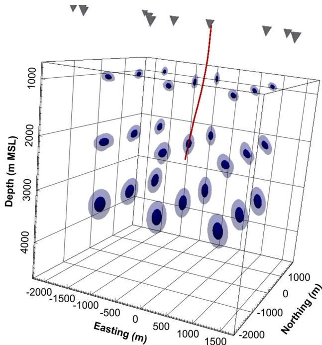
**Figure 6.** 3-D view of the relocation uncertainties at 68.3 per cent (dark blue) and 99.7 per cent (light blue) confidence levels of 27 sources distributed around GRT1 well (red curve). Part of the seismic stations is also displayed (grey cones).
