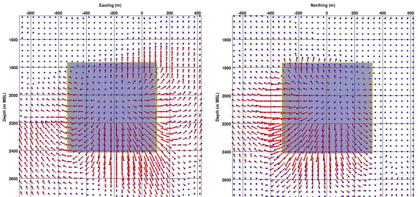
**Figure 12.** Projection of the initial locations and of the relocations of the synthetic earthquake hypocentres for the vertical E–W plane (left) and for the vertical N–S plane (right). The relocated hypocentres (blue points) should be shifted along the red line to come back to their initial location. The shadowed area represents the perturbed velocity zone.
