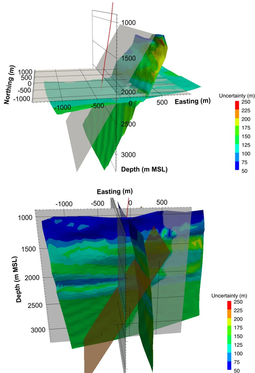
**Figure 14.** 3-D view of the relocation of the synthetic events initially located on the horizontal plane and along the fault (top) and on the N–S and E–W vertical plane (bottom). The initial locations were on the grey planes whereas the relocations are on the coloured planes. The colour scale is associated with the largest uncertainty value which varies between 50 and 250 m. The location of the fault is shown by the brown plane (bottom).
