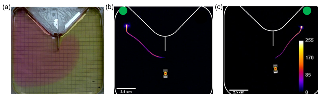
Figure 1. a) \nabla\text{pH} revealed by a universal pH indicator 30 s after the beginning of acid injection from the upper left corner. b) Trajectory of the light-emitting swimmer recorded in the dark in the presence of a \nabla\text{pH} originating from the upper left corner. c) Same as (b) but with acid injection from the upper right corner. The green dot represents the source of acid; the color scale codes the light intensity and a swimmer symbol is positioned at the initial launching location.
