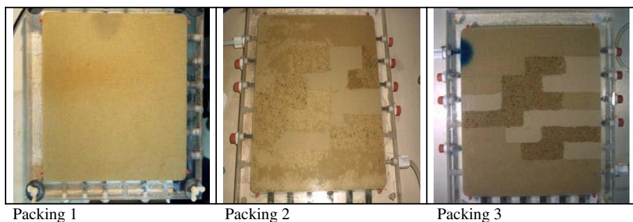
Fig. 1. Sand packing arrangements used for the laboratory experiments. Packing 1: homogeneous packing with medium sand. Packing 2: heterogeneous packing arrangement with coarse, medium and fine sand. Packing 3: heterogeneous packing arrangement with coarse, medium and fine sand.
