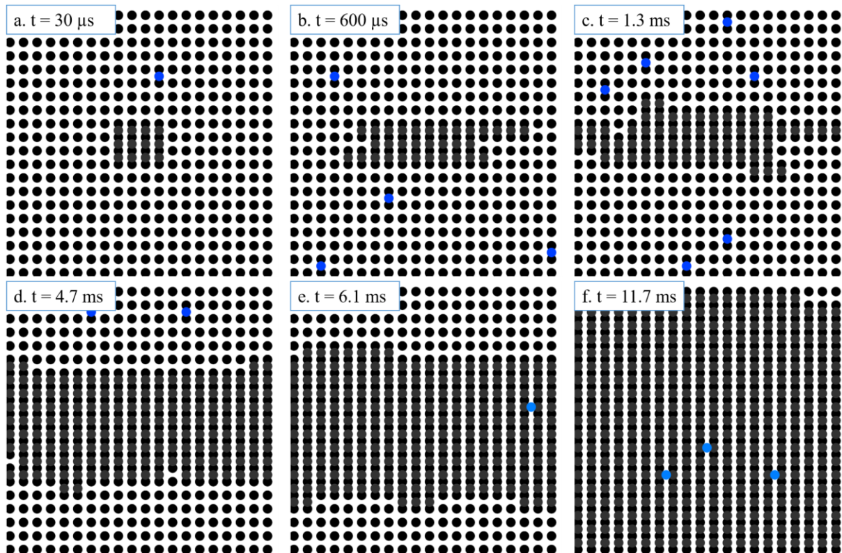
Figure 5. Growth of a single diamond layer (top view), for a temperature of 850°C, 4% methane concentration in the gas phase and a couple pressure/microwave power set to 200 mbar/3 kW.
