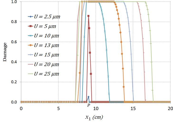
Figure 11: Damage distribution along the notch axis
