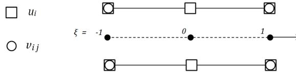
Figure 16: Second gradient cohesive interface element (parent element)
