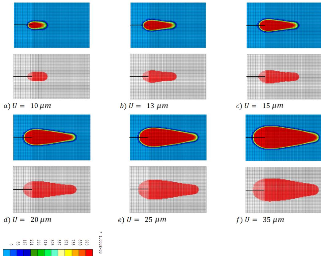
Figure 8: Damage distribution and loading integration points for different levels of loading
