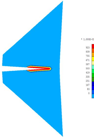
Figure 24: Mode I crack propagation test revisited : Damage distribution for  $U = 25\mu\text{m}$
