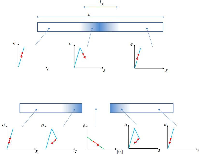
Figure 19: Continuous - discontinuous transition in the 1D case
