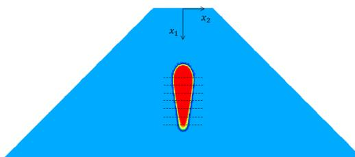
Figure 9: Damage distribution for  $U = 20 \mu m$
