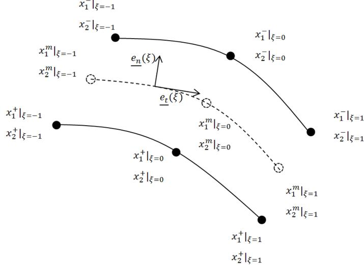
Figure 17: Geometrical interpolation and local coordinate system
