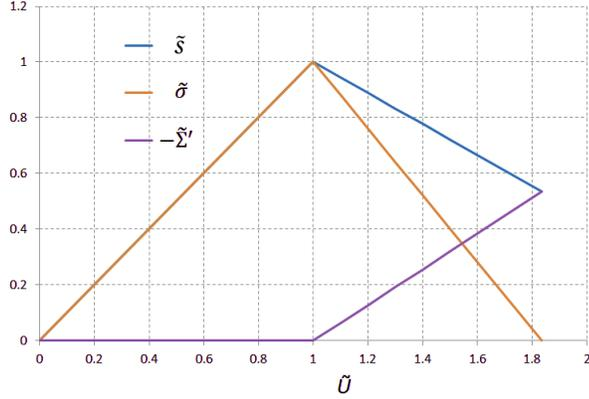
Figure 4: One-dimensional tensile test : Adimensionalized tensile traction  $\tilde{s}$ , stress  $\tilde{\sigma}$  and  $-\tilde{\Sigma}'$  evolutions at the point of maximum strain with  $\omega = 13.7m^{-1}$  and  $\eta = 9.7m^{-1}$
