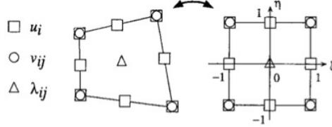
Figure 15: 2D second gradient finite element, [18], [59].
