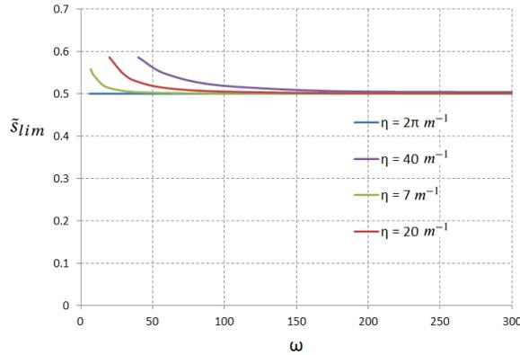
Figure 5: One-dimensional tensile test : Evolution of  $\tilde{s}_{lim}$  as a function of  $\eta$  and  $\omega$  ( $L = 1m$ )
