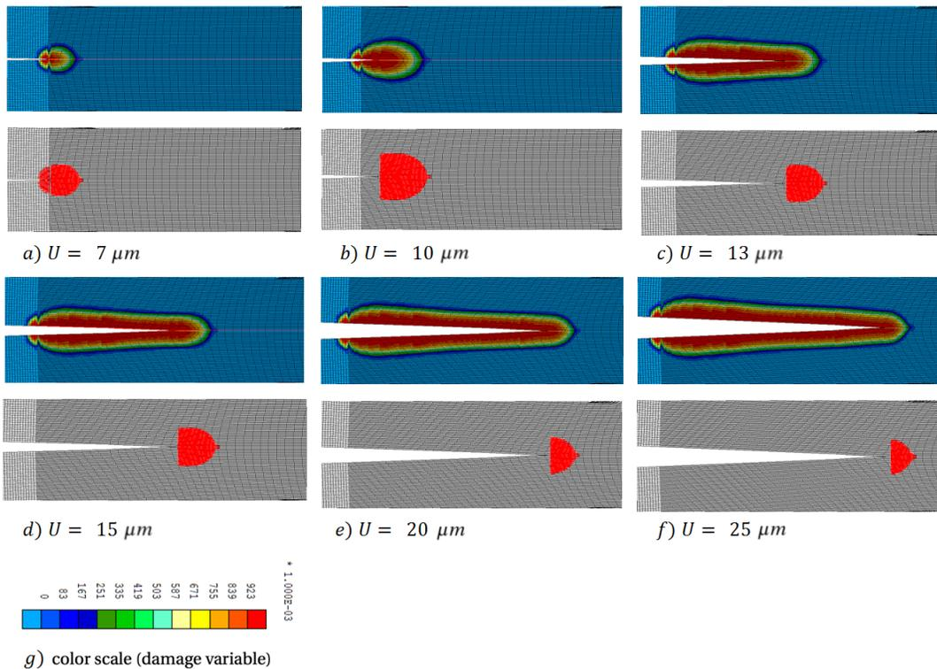
Figure 25: Mode I crack propagation test revisited: Damage distribution and loading integration points
