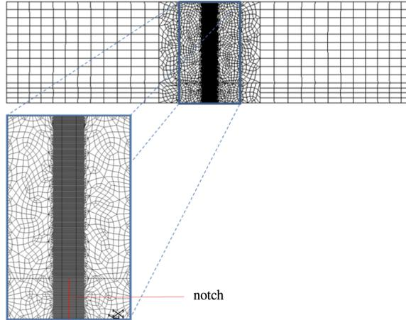
Figure 28: 3 points bending test: Finite element mesh
