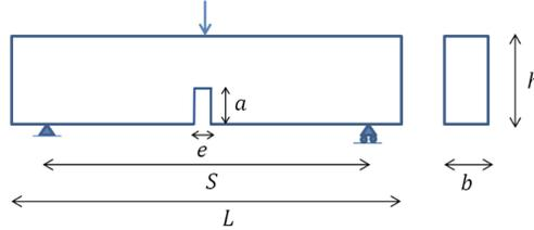
Figure 26: 3 points bending test: Geometry (see also Table3)
