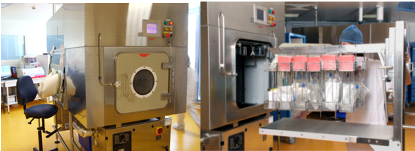
Figure 6.2. Isolator (left) and part of the sterilizer carrying the baskets (right). For a color version of the figure, please see www.iste.co.uk/sarazin/health.zip
