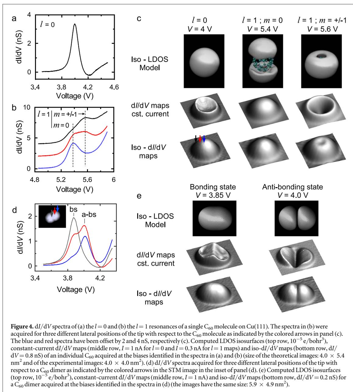
top part of the molecule is imaged. This is a direct consequence of the sphericity of  $C_{60}$ , showing that constant-height measurements produce limited results for a corrugated surface.
