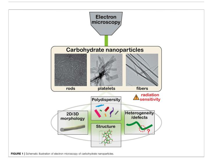
choice for the characterization of various structural and morphological aspects at the nanoscale (**Figure 1**), although the intrinsic radiation sensitivity and electron transparency of carbohydrate solids have often hindered the in-depth investigation by TEM. Many researchers have contributed to the EM of carbohydrate crystals in attempts to reveal their ultrastructural details, as reviewed elsewhere (Chanzy and Vuong, 1985; Ogawa et al., 2019).
