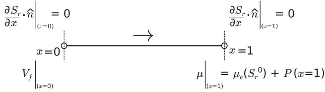
**Fig. 3.** Schematic of the imbibition simulations showing boundary conditions applied on the one-dimensional domain. The arrow indicates the direction of motion of the self-similar interface. The form of natural boundary condition  $V_f(x=0)$  is given in Eq. (43).
