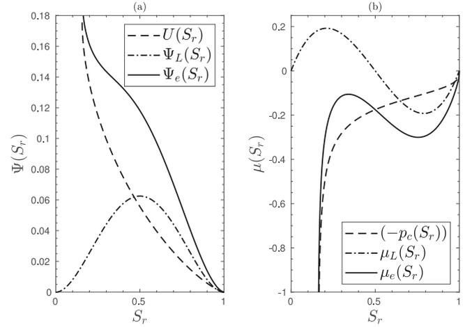
Fig. 1. (a) Energy densities,  $\Psi_e(S_r)$ ,  $\Psi_L(S_r)$ ,  $U(S_r)$ ; (b) chemical potentials,  $\mu_e(S_r)$ ,  $\mu_L(S_r)$ ,  $p_c(S_r)$ . All functions plotted are dimensionless according to the scheme presented in Section 2.2.7.
