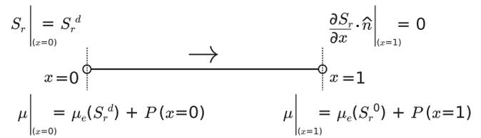
Fig. 6. Schematic of the drainage simulations showing boundary conditions applied on the one-dimensional domain for  $t > t_d$ . The arrow indicates the direction of motion of the self-similar interface.
