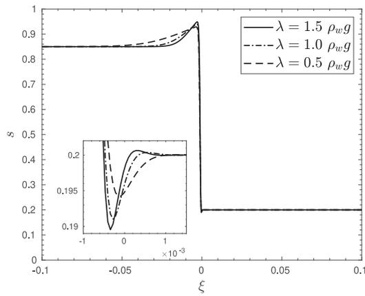
Fig. 16. TW-solutions of Eq. (48) representing imbibition for  $\lambda = 0.5\rho_w g, \rho_w g, 1.5\rho_w g$ , with boundary conditions  $s_+ = 0.20, s_- = 0.85$ ; Solutions are shown in a restricted range of  $\xi$  for clarity.
