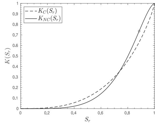
**Fig. 2.** Relative permeability functions  $K(S_r)$ , Eq. (39), for different values of van Genuchten parameters ( $a, b, c$ ).  $K_C$ :(1.175, 0.85, 2.0),  $K_{NC}$ :(8.0, 2.0, 0.5). Inflection point is shown as a circle on curve  $K_{NC}(S_r)$ .
