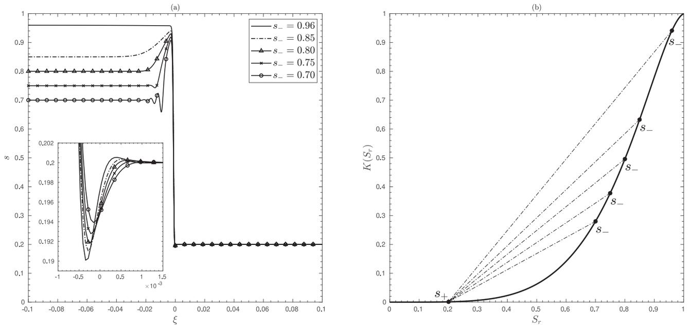
Fig. 11. (a)TW-solutions of Eq. (48) for  $\lambda = \rho_w g$ , with boundary conditions  $s_+ = 0.20$ ,  $s_- = 0.96, 0.85, 0.80, 0.75, 0.70$ . Solutions are shown in a restricted range of  $\xi$  for clarity. (b) the corresponding connections shown on the curve  $K(S_r)$ .
