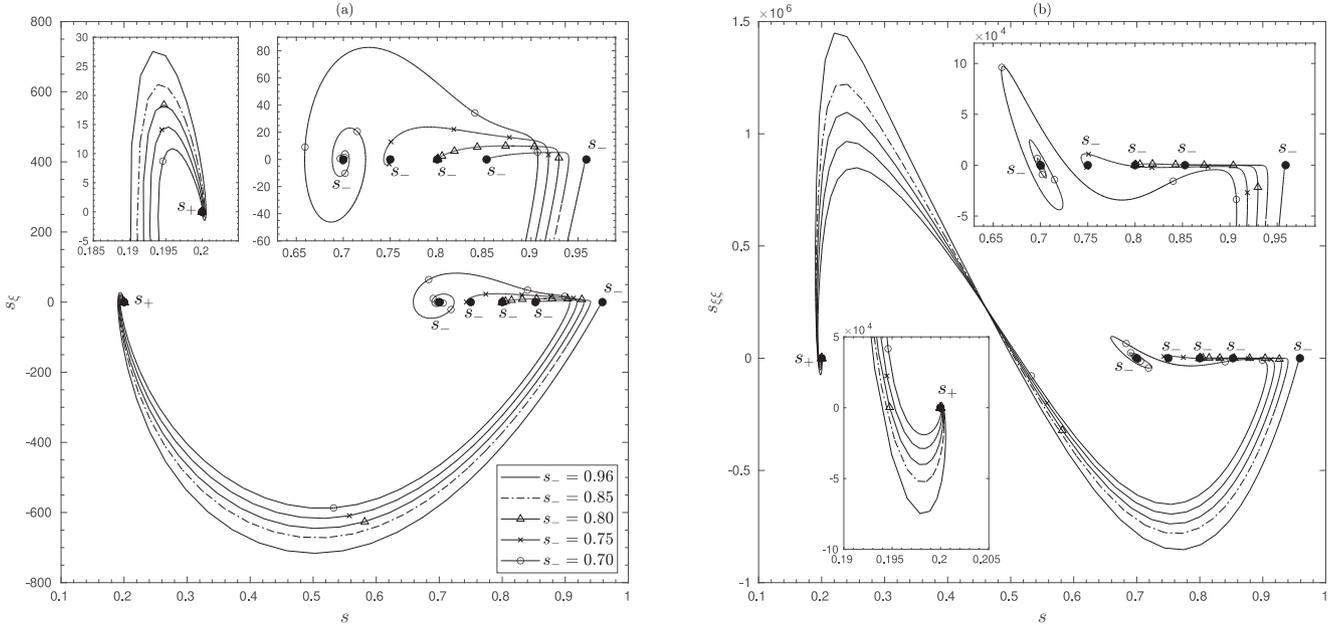
Fig. 12. TW-solutions shown as trajectories in the phase space defined by of Eq. (49) for  $\lambda = \rho_w g$ , with boundary conditions  $s_+ = 0.20$ ,  $s_- = 0.96, 0.85, 0.80, 0.75, 0.70$ ; phase plane views (a)  $(s, s_\xi)$ , (b)  $(s, s_{\xi\xi})$ .
