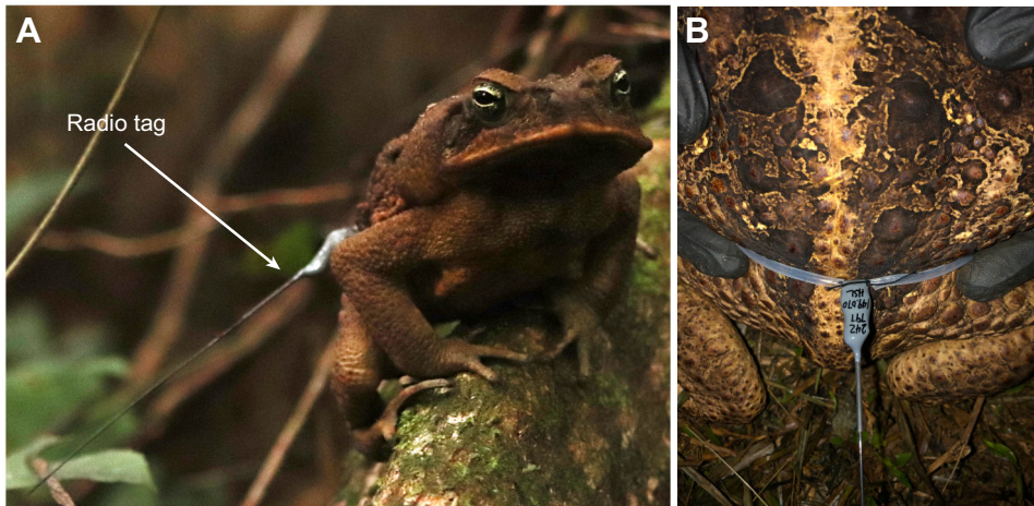
Fig. 1. Rhinella marina toads tagged with radio transmitters. (A) A male toad with an attached radio transmitter. (B) Close up of a radio transmitter attached to a toad's waist with a belt of silicone tubing.
