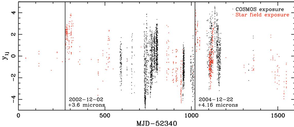
**Fig. B.9.** Temporal variation of the first principal component coefficient  $y_{1j}$ , which is related to the HST focus position, measured in the stellar field and COSMOS exposures. The long-term shrinkage of the OTA is well visible as a decrease in the mean  $y_{1j}$ , which was compensated with the marked focus adjustments. The wide spread at a given date is not caused by measurement errors but orbital breathing leading to substantial short-term focus variations.
