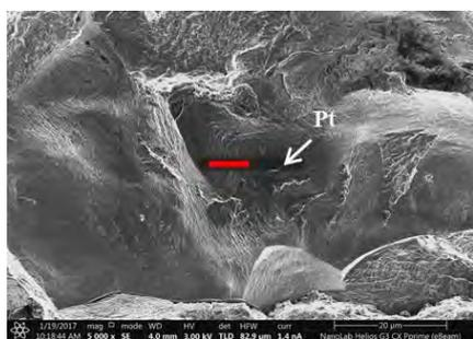
(b-1) SEM image of the first position of fracture surface.
