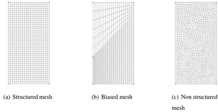
Figure 20: Biaxial test: three different types of mesh
