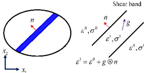
Figure 2: Principle scheme of a shear band
