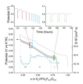
Figure 11: Continuous galvanostatic charge performed at a rate of C/50 followed by a discharge performed in GITT conditions for KVPO<sub>4</sub>F<sub>0.5</sub>O<sub>0.5</sub> (at a rate of C/50, with steps of 15 minutes ( $\Delta x = 0.005$ ) and relaxation time until the slope dE/dt is inferior to 1 mV·h<sup>-1</sup>).
