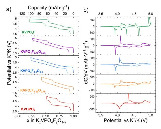
Figure 10: a) Galvanostatic curves (2<sup>nd</sup> cycle) obtained for all materials in K metal half-cells at C/20. b) Corresponding derivative curves.
