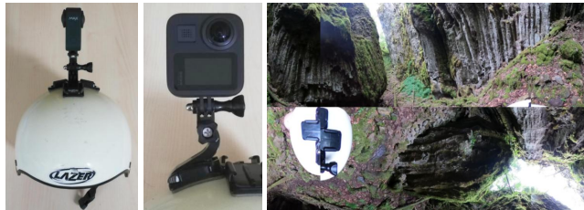
Fig. 1. A Gopro Max 360 camera and a cubemap image.
