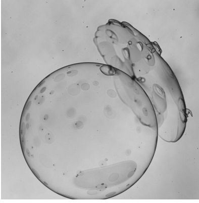
Figure 12. Closed bubble and freely floating film sheet, not in contact with each other. The islands in the bubble remain undistorted, while those in the floating film form bulges under comparable conditions. Image size 4 mm \times 4 mm.
