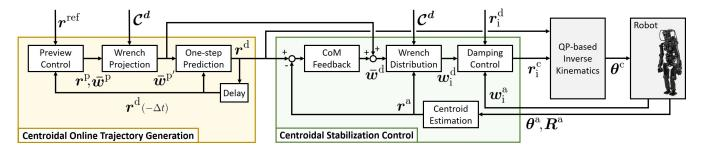
Fig. 1. Overall components of the control system for humanoid multi-contact motion.
