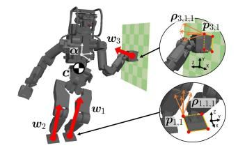
Fig. 2. Contact constraints in wrench distribution.
