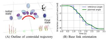
Fig. 8. Centroidal trajectory generation of cartwheel motion.
