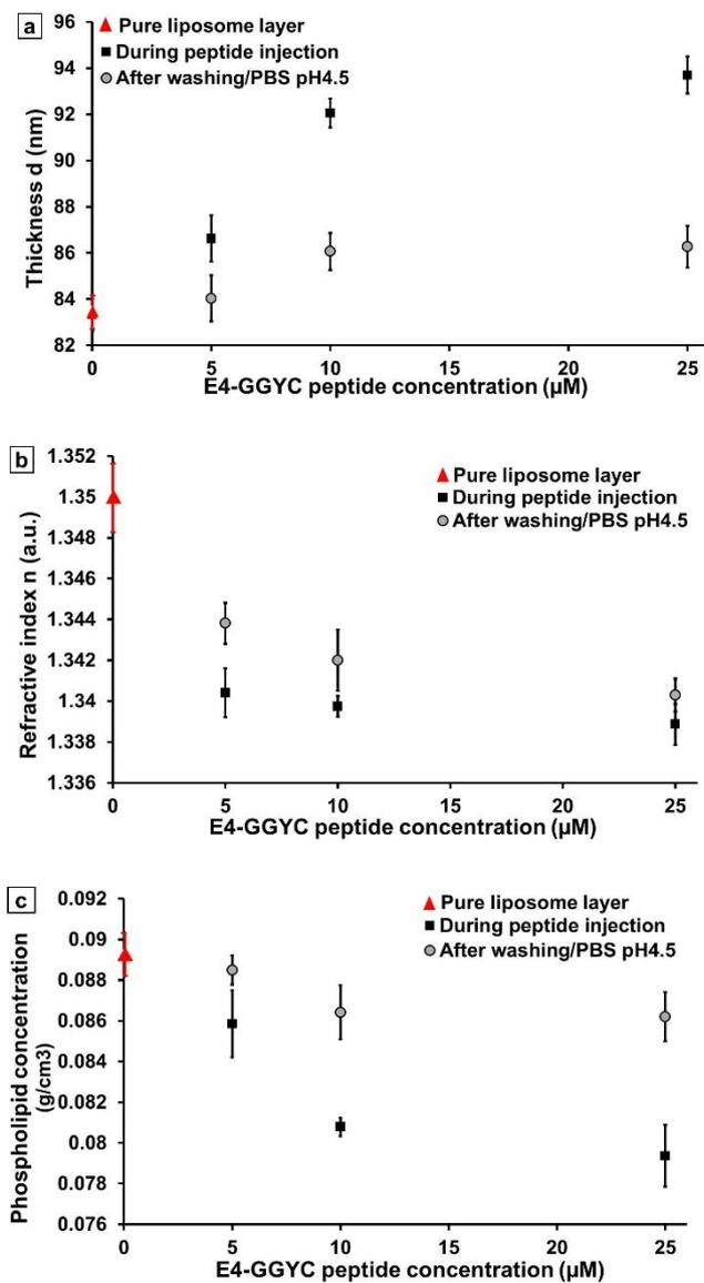
**Figure 4.** Effect of 5-25  $\mu\text{M}$  E4-GGYC injection on the thickness  $d$  (a), refractive index  $n$  (b) and concentration of phospholipids  $C_p$  (c) of the immobilized liposome layer at pH 4.5, before and after the washing step in PBS, pH 4.5.
