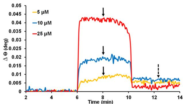
**Figure 2.** Superimposed sensorgrams (normalized peak angular position vs time) recorded during injection of 5–25  $\mu\text{M}$  E4-GGYC peptide at pH 4.5 on the liposome-functionalized surface. The arrows indicate the positioning for  $d$  and  $n$  calculations (Table 3) at 670 nm.
