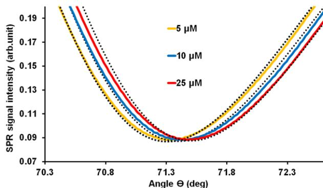
**Figure 3.** SPR peak full angle scans measured at 670 nm of the liposome-supported surfaces after injection of 5–25  $\mu\text{M}$  E4-GGYC solutions at pH 4.5 (solid curves), with corresponding fits from LayerSolver™ modeling (dotted curves). The SPR curve corresponding to each concentration was taken at the equilibrium of peptide/liposome interaction for the modeling by LayerSolver™ software.
