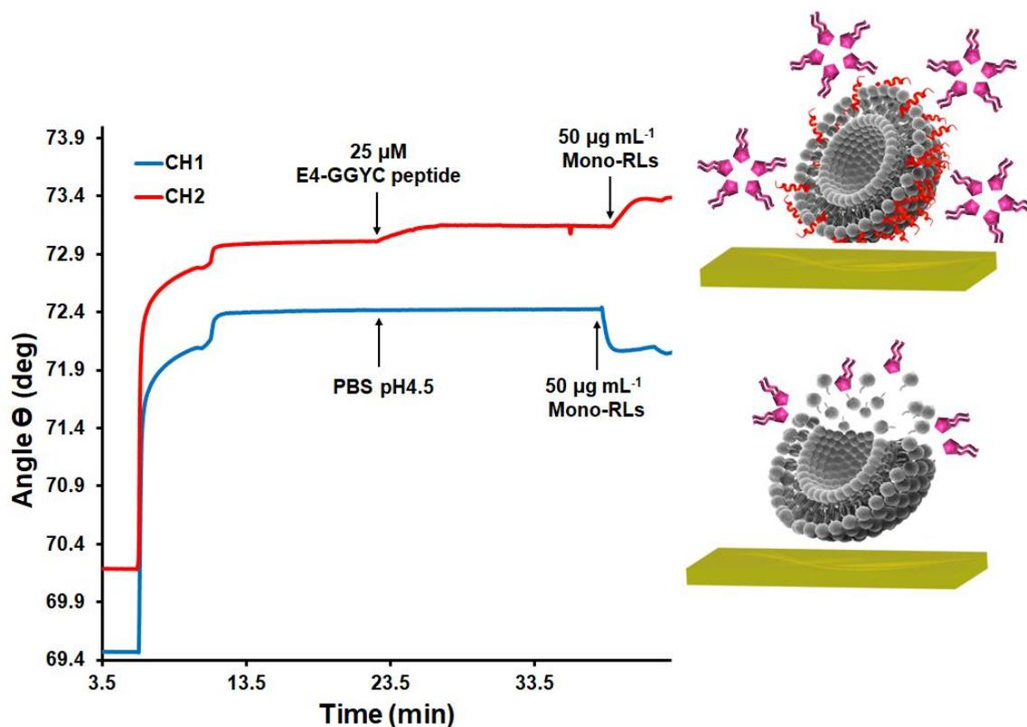
**Figure 8.** Sensorgrams measured in PBS pH 4.5 and at 670 nm wavelength during mono-RL injection at a concentration of 50  $\mu\text{g}/\text{mL}$  on a pure liposome layer (CH1) and on a liposome layer saturated with 25  $\mu\text{M}$  of E4-GGYC peptide at pH 4.5 (CH2) .
