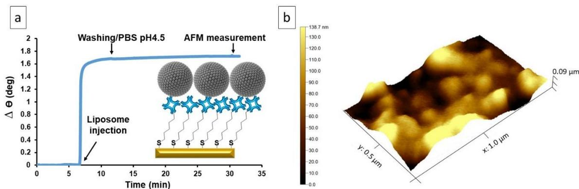
**Figure 1.** MP-SPR sensorgram of the liposome adsorption on a streptavidin functionalized surface before AFM measurement (a), and AFM topographic image by tapping-mode of the liposome-functionalized surface (b).
