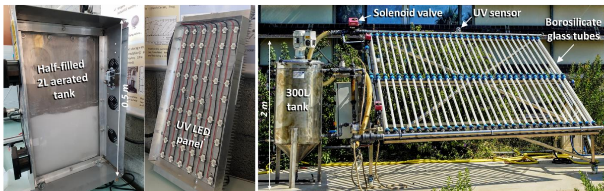
227 228 Figure 2: Experimental set up of the artificial light photoreactor (left) & the natural sunlight one (right). 229
