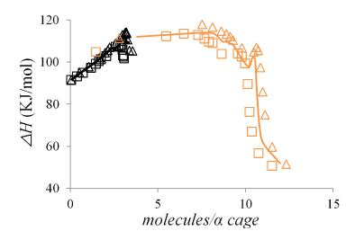
**Figure 7.** (color online) Simulated isosteric adsorption enthalpies for xylene isomers at 175°C in bulk BaX zeolite (black) and in a BaX zeolite with an external surface (orange). The data for pure xylene isomers corresponds to the different symbols: px (triangles) and mx (squares). The adsorption enthalpy for an equimolar px/mx mixture is indicated by the solid line.
