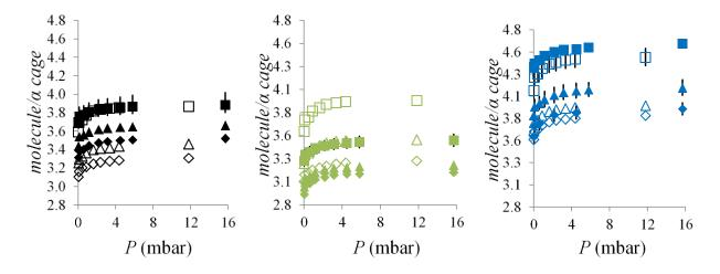
**Figure 1.** (color online) Single component adsorption isotherms for px and ox in hierarchical and conventional BaX zeolites: Conventional (black), LL (green) and NA-3 (blue). Filled symbols correspond to px adsorption while empty symbols correspond to ox adsorption. The temperatures are indicated by the symbols: squares (100°C), triangles (150°C) and diamonds (175°C).
