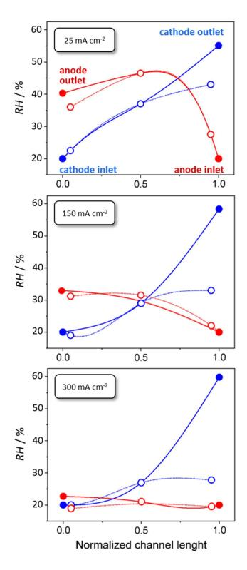
**Figure 8.** Evolution of the RH distribution along the anode (red) and cathode (blue) gas flow paths with the current density (reported in the legend) in the FC operated at T = 32°C. Full symbols correspond to direct measurements at the FC inlets and outlets whereas open symbols are RH values deduced from the membrane surface water content as given by  $\mu$ -Raman.
