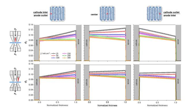
**Figure 3.** Comparison of the evolution of the membrane inner water distribution with the current density (reported in the legend) at the different probed positions (top: channel, bottom: lands, left: cathode inlet, middle: center, right: cathode outlet) in the cell operated at  $T_{\text{room}}$ .
