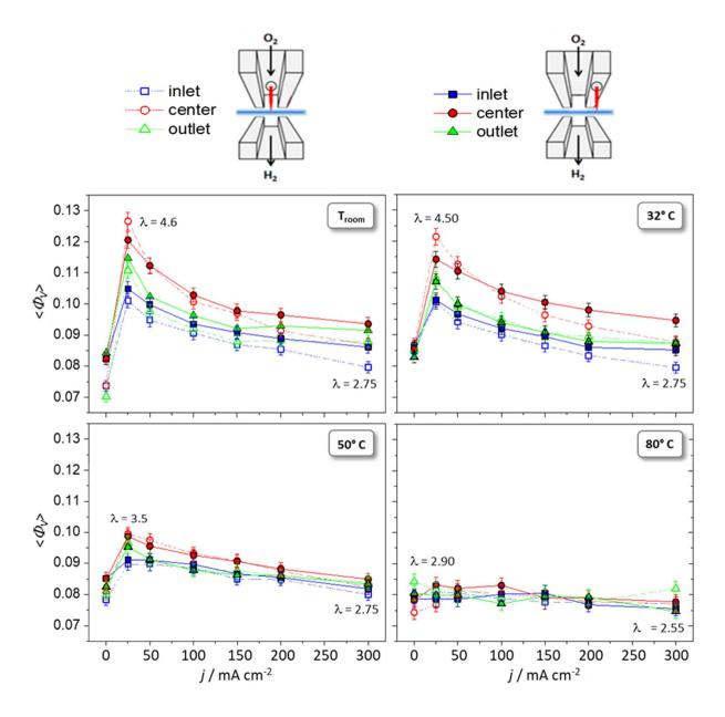
**Figure 5.** Evolution with the current density of the membrane average water volume fraction at the channel (open symbols) and under-lands (full symbols) positions in the cell operated at different T. The minimum and maximum water contents measured for a given T are also reported as hydration number  $\lambda = [H_2O]/[SO_3]$ .
