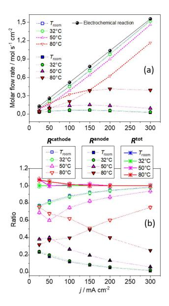
**Figure 6.** (a) Evolution with current of the extra water flows measured at the cathode (open symbols) and anode (full symbols) sides (the evolution of the overall flow of the electrochemically produced water is also reported in full black symbol; errors are inside the symbol size) and of (b) the ratios between the extra water flow measured at each electrode and the overall extra water, at the different FC operating T (reported in the legend).
