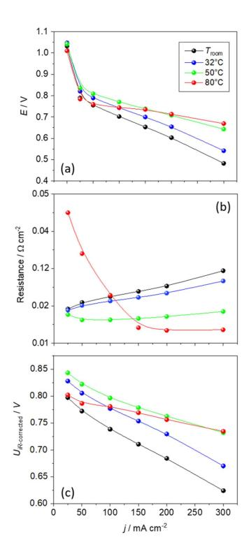
**Figure 2.** (a) FC polarization curves at different operating T (reported in the legend) and corresponding evolutions of (b) the ohmic resistance and (c) the iR corrected potential as a function of the delivered current.
