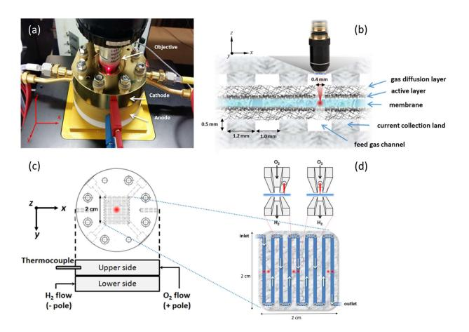
**Figure 1.** (a) The PEMFC for operando Raman microspectroscopy measurements. (b) Schematic side view of the Raman probed position at the gas distribution channel. (c) Schematic top view of the bipolar plate with the carved single serpentine gas distribution channel. (d) In scale schematic representation of the configuration of the gas distribution channel and positions probed by the Raman exciting radiation.
