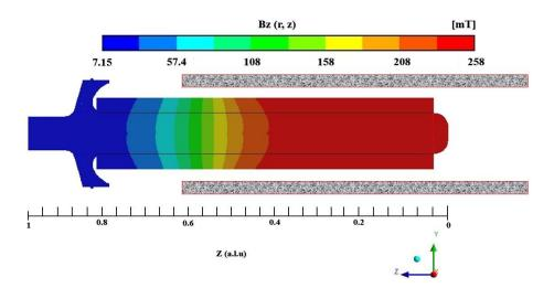
Figure 6 – Field of the axial component of the magnetic field
