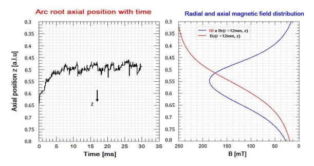
Figure 9 – Arc root axial position versus time in the left and, in the right radial (in blue) and axial (in red) external magnetic field components. I=260A, D=0.037kg/s.
