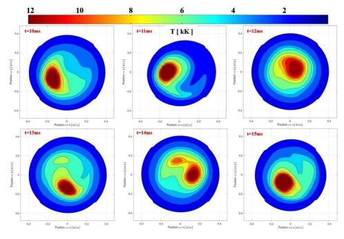
Figure 15 – Temperature fields at the exit plane from 10 to 15ms (step 1ms)
