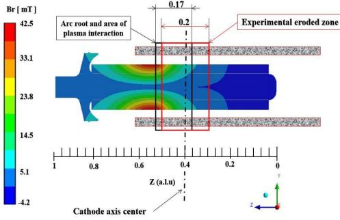
Figure 10 – Wear position: experiment and model
