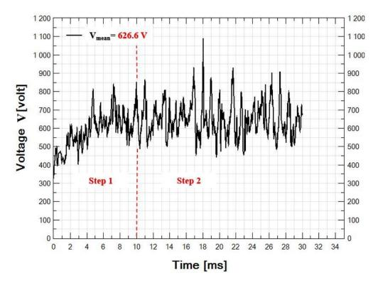
Figure 8 – Electric arc voltage versus time
