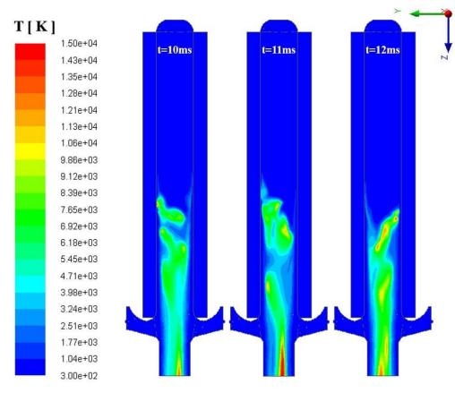
Figure 14 – Temperature fields in the hallow cathode (t=10, 11 and 12ms)
