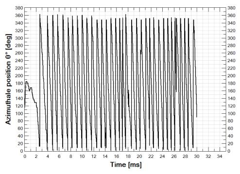
Figure 11 – Arc root azimuthal position versus time
