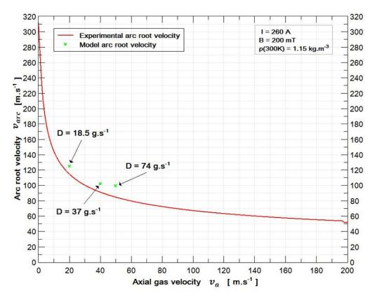
Figure 13 – rotational arc root velocity versus axial gas velocity
