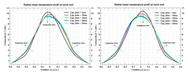
**Figure 17** – Mean temperature profiles integrated on time at the exit plane for different integrated times on two perpendicular directions.
