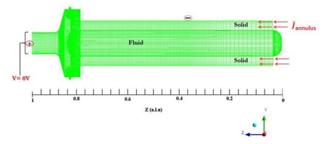
Figure 2 – Domains studied (Solid and Fluid) and grid
