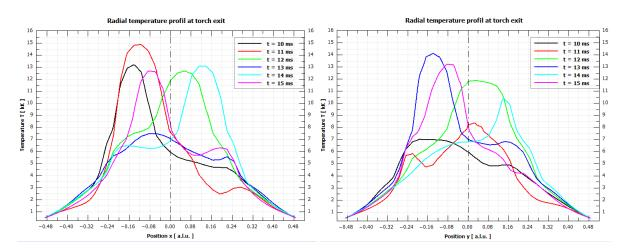
Figure 16 – Temperature profiles at the exit plane for different times on two perpendicular directions.
