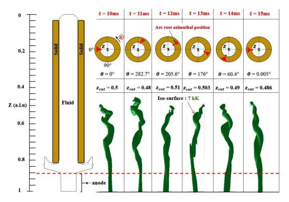
Figure 7 – Arc behavior within the geometry
