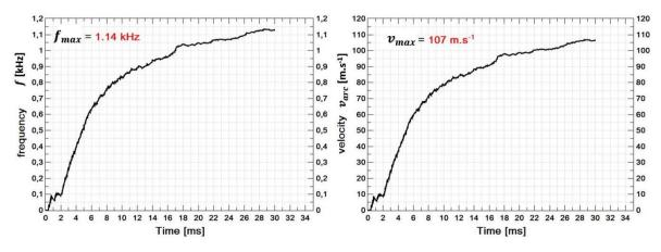
Figure 12 – Arc frequency and velocity versus time
