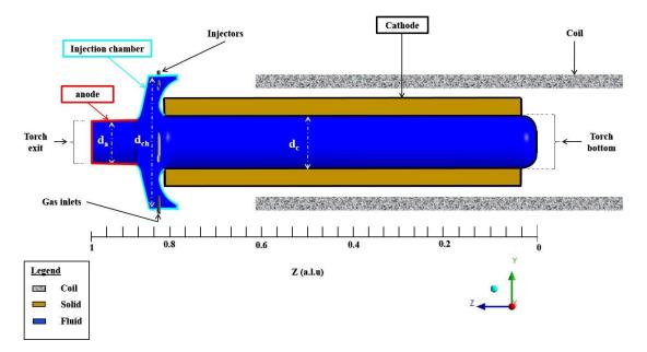
Figure 1 – Overview of the studied device including the simplified scheme and position of the coil
