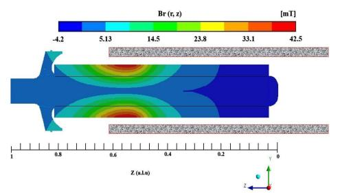
Figure 5 – Field of the radial component of the magnetic field
