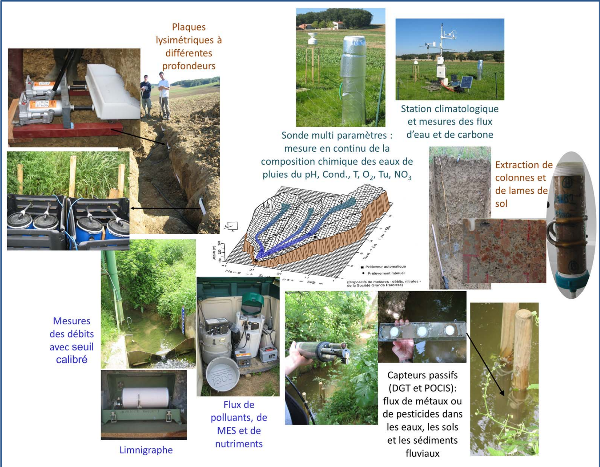
Figure 8- The instrumentation installed on the Auradé Catchment for monitoring of the different compartments : soil solution (top left), rain water and climatological station (top right), soil experiments (middle right), stream water (bottom) with water height and discharge, automatic sampler, multi parameter probe with different sensors, DGT and POCIS passive samplers (from left to right).
