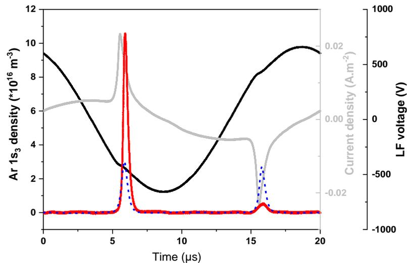
*Figure 4. Number density of Ar  $1s_3$  atoms close to the upper electrode (solid) and in the middle of the gap (dash) over a complete cycle of the low frequency excitation (LF 650V, 50 kHz). Applied voltage (black) and total current density (grey, discharge + displacement current density) are also shown for comparison. On first half cycle of the applied voltage, the upper electrode is cathode while on the second half-cycle, the lower electrode is cathode.*
