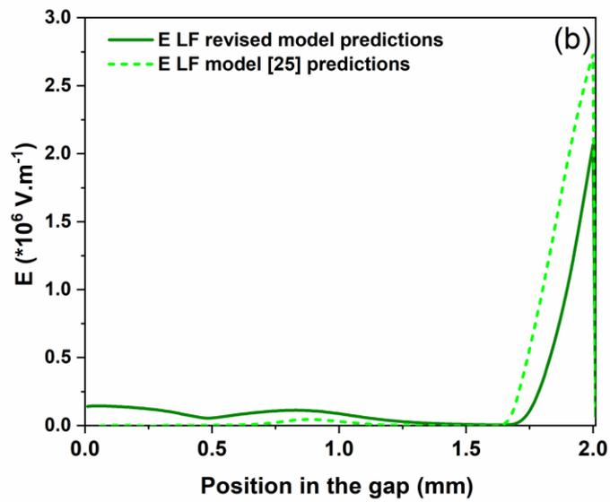
Figure 6. a)  $Ar(1s)$  number density evolution over space and time in the LF DBD, b) spatial profile of the electric field along the gap when  $Ar(1s)$  is maximum at the anode (vertical line in a). In b), the results for the electric field are shown with the model used in [25] and with the revised version developed in this work.
