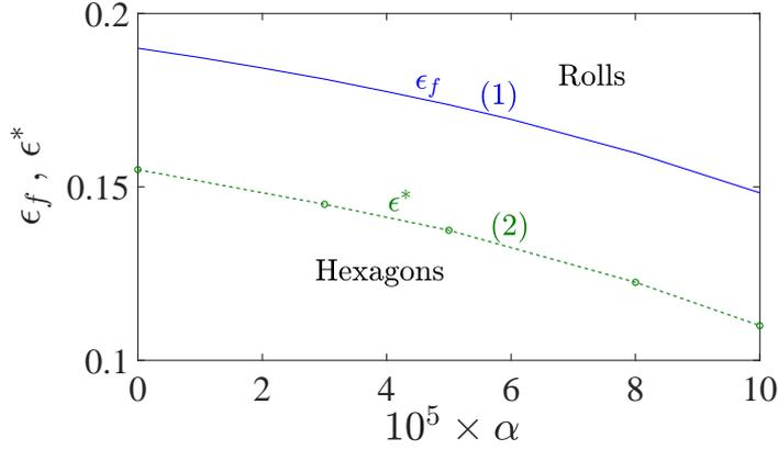
FIGURE 26. Threshold for hexagon-roll transition in the case where there is no distortions of hexagons as a function of the shear-thinning degree, with  $q = 0.55$ ,  $r = 2.5$  and  $\text{Pr} = 50$ . (1) Curve of equal energy for hexagons and rolls, (2) numerical simulations.
