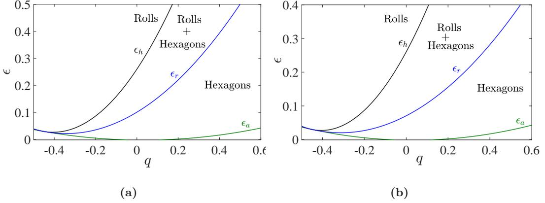
FIGURE 14. Amplitude stability curves in  $(\epsilon, q)$  plane, at  $r = 2.5$ ,  $\text{Pr} = 50$  and two different values of  $\alpha$ : (a)  $\alpha = 0$  Newtonian fluid, (b)  $\alpha = 10^{-4}$  Carreau fluid.
