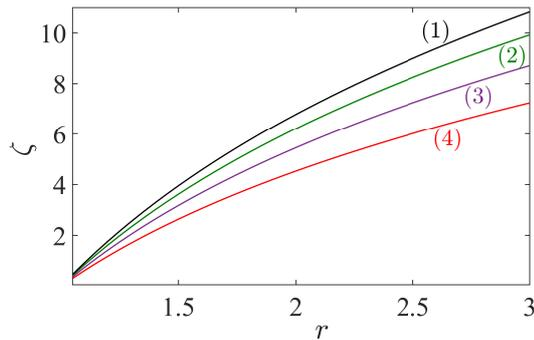
FIGURE 9. Variation of  $\zeta$  with the ratio viscosity  $r$  for different values of the Prandtl number.
