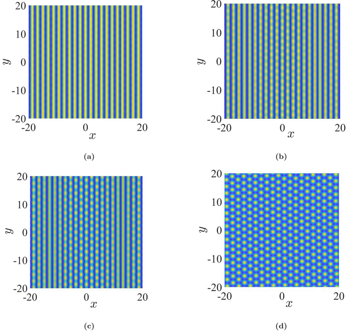
FIGURE 25. Initial condition ( $\mathcal{P}_3$ ): rolls with  $q = 0.25$ ,  $\epsilon = 0.1$ ,  $r = 2.5$ ,  $\alpha = 10^{-4}$  and  $\text{Pr} = 50$ . The reconstructed vertical velocity  $w$  is shown at different times: (a)  $t = 0$ , (b)  $t = 11$ , (c)  $t = 15$  and (d)  $t = 2000$ .
