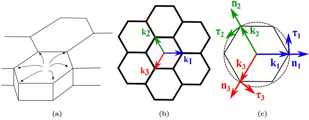
FIGURE 3. (a) Hexagonal convection with flow up in the center. (b) Basic wave vectors of hexagonal pattern. (c) Unit vectors:  $\mathbf{n}_i$  parallel and  $\boldsymbol{\tau}_i$  perpendicular to the wave vector.
