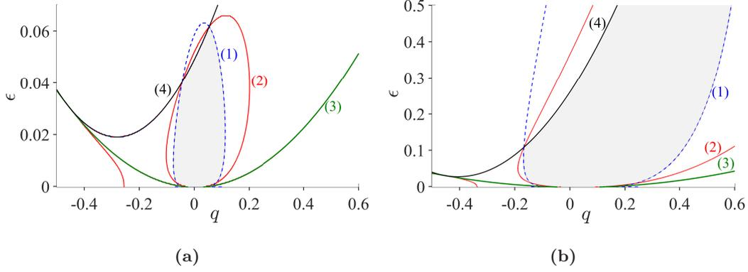
FIGURE 17. Hexagon stability diagram for a Newtonian fluid at  $\text{Pr} = 50$  and two different values of the viscosities ratio: **(a)**  $r = 1.5$  and **(b)**  $r = 2.5$ . Hexagons are stable inside the gray area. Curve (1):  $D_{\perp} = 0$ , curve (2)  $D_{\parallel} = 0$ , curve (3) bifurcation from the conductive state to convection with hexagons, curve(4) bifurcation from hexagons to rolls.
