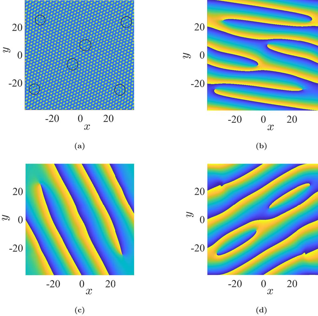
FIGURE 23. Initial condition ( $\mathcal{P}_1$ ): hexagons with  $q = 0.45$ ,  $\epsilon = 0.1$ ,  $r = 2.5$ ,  $\alpha = 10^{-4}$  and  $Pr = 50$ . **(a)** Contours of the vertical velocity  $w = \sum_{i=1}^3 A_i \exp(i\mathbf{k}_{c,i} \cdot \mathbf{x}) + c.c.$  at  $t = 1000$ ; **(b)** phase of  $A_1$ ; **(c)** phase of  $A_2$  and **(d)** phase of  $A_3$ .
