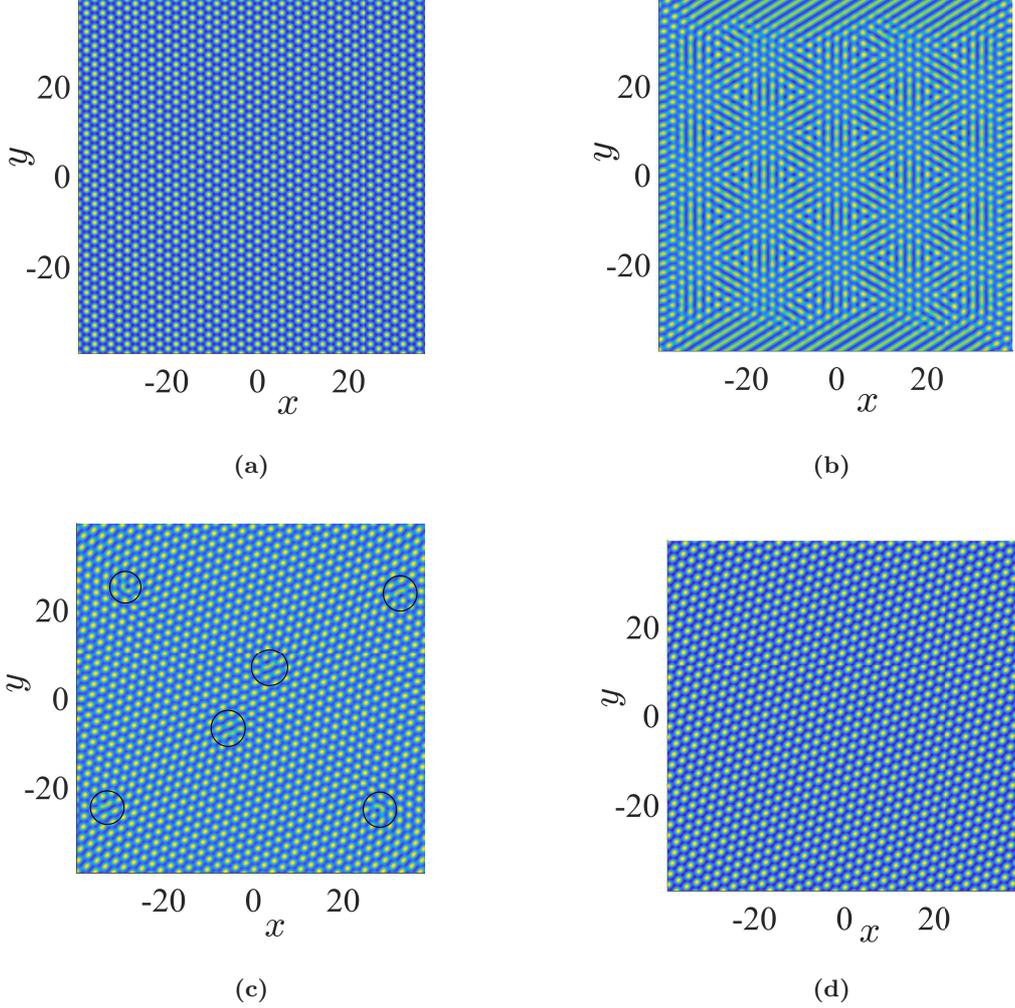
FIGURE 21. Initial condition ( $\mathcal{P}_1$ ): hexagons with  $q = 0.45$ ,  $\epsilon = 0.1$ ,  $r = 2.5$ ,  $\alpha = 10^{-4}$  and  $\text{Pr} = 50$ . Contours of the vertical velocity  $w = \sum_{i=1}^3 A_i \exp(i\mathbf{k}_{c,i} \cdot \mathbf{x}) + c.c.$  for a hexagonal pattern undergoing the transverse instability. The contours are shown at times (a)  $t = 0$ ; (b)  $t = 10$ ; (c)  $t = 1000$  and (d)  $t = 2000$ . In the panel (c), the penta-hepta defects are circled.
