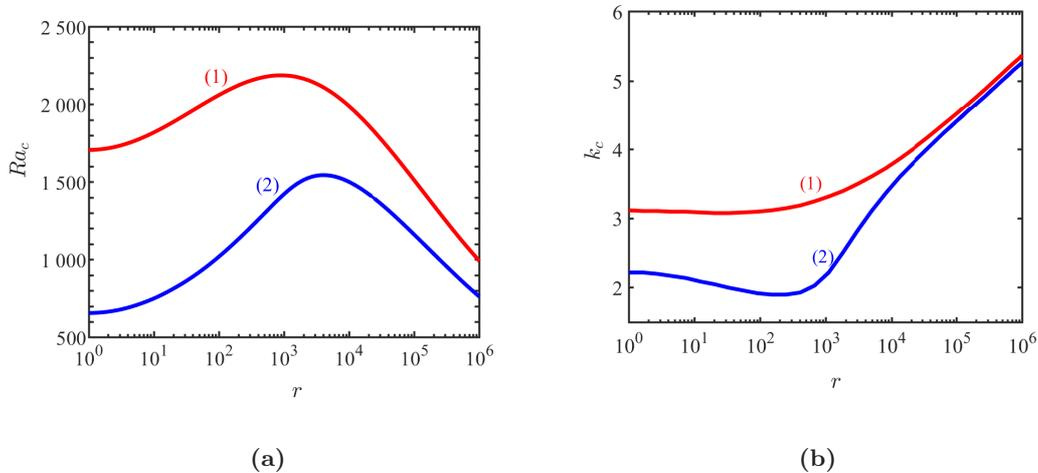
FIGURE 1. Exponential fluid. Critical Rayleigh number **(a)** and critical wavenumber **(b)** as function of the viscosity ratio. (1) NSBC, (2) SFBC.
