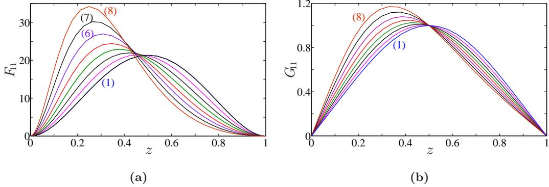
FIGURE 2. Exponential fluid. **(a)** Vertical velocity eigenfunction and **(b)** temperature perturbation at the first order as function of the depth  $z$  for different values of the thermodependency coefficient  $c$ . (1)  $c = 0$ ; (2)  $c = 1$ ; (3)  $c = 2$ ; (4)  $c = 3$ ...increasing  $c$  by step 1 until curve (8)  $c = 7$ .
