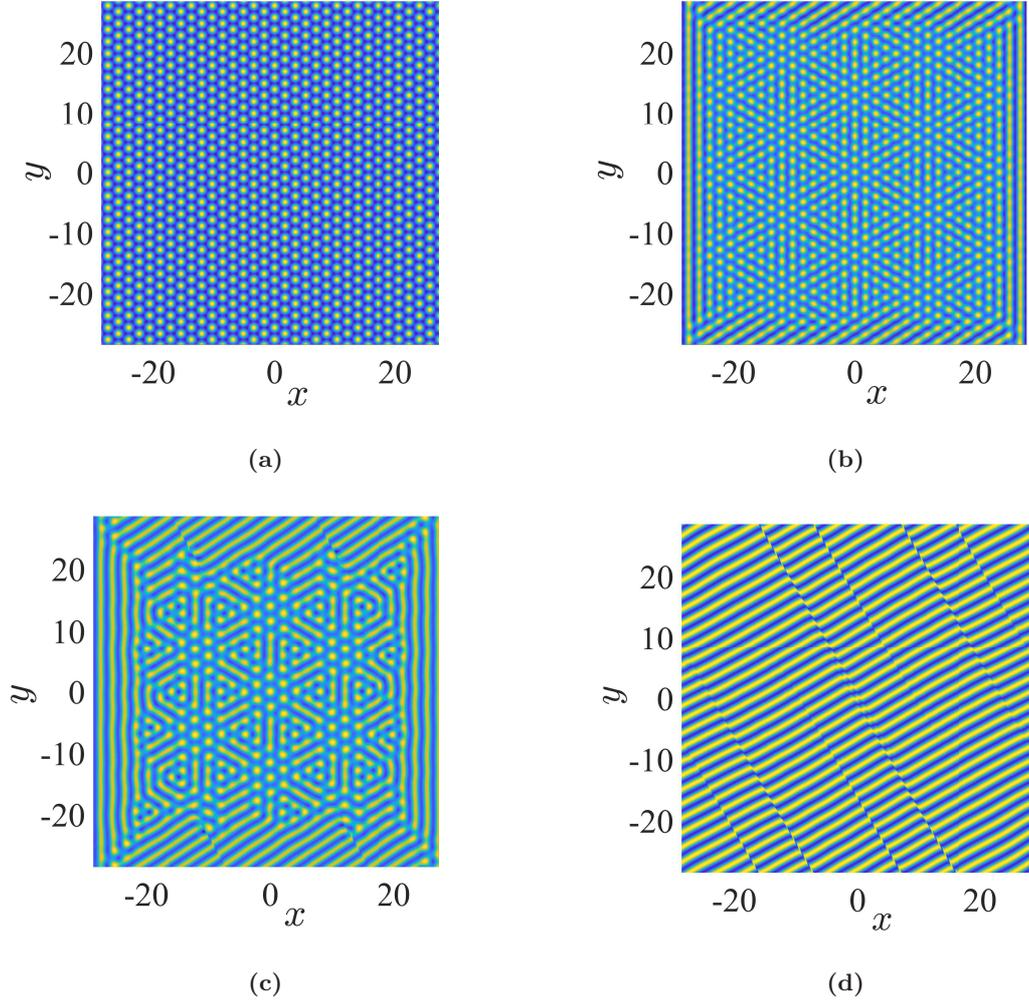
FIGURE 24. Initial condition ( $\mathcal{P}_2$ ): hexagons with  $q = 0.55$ ,  $\epsilon = 0.3$ ,  $r = 2.5$ ,  $\alpha = 10^{-4}$  and  $\text{Pr} = 50$ . The reconstructed vertical velocity  $w$  is shown at different times: (a)  $t = 0$ , (b)  $t = 2$ , (c)  $t = 10$  and (d)  $t = 100$ .
