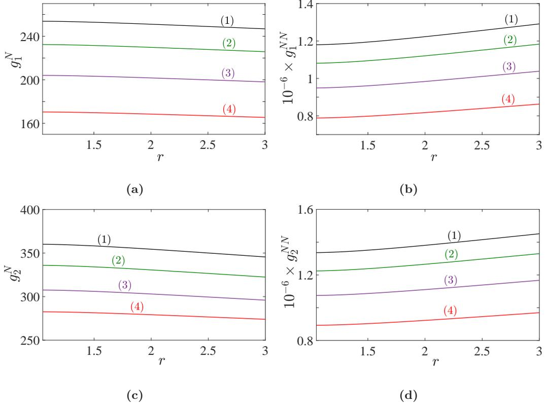
FIGURE 10. (a) “Newtonian” and (b) non-Newtonian contribution to the first Landau coefficient and to the cross-saturation coefficient (c) and (d) respectively as a function of  $r$  for different values of Pr. (1) Pr = 50; (2) Pr = 5; (3) Pr = 2; (4) Pr = 1.
