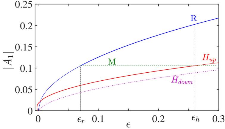
FIGURE 15. Bifurcation diagram for hexagons in the case where  $g_2 > g_1$  with the parameters  $r = 2.5$ ,  $q = 0$  and  $\alpha = 10^{-4}$ . The amplitude  $|A_1|$  is plotted against the distance to the threshold  $\epsilon$ , for the roll-solution branch (labeled  $R$ ), for the mixed mode branch (labeled  $M$ ) and for the two hexagon-solution branches, up- and down-hexagons. Solid lines indicate stable solutions and dashed lines represent unstable solutions.
