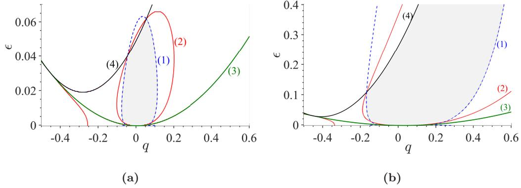
FIGURE 18. Hexagon stability diagram for a shear-thinning fluid with  $\alpha = 10^{-4}$  at  $\text{Pr} = 50$  and two different values of the viscosities ratio: **(a)**  $r = 1.5$  and **(b)**  $r = 2.5$ . Hexagons are stable inside the gray area.
