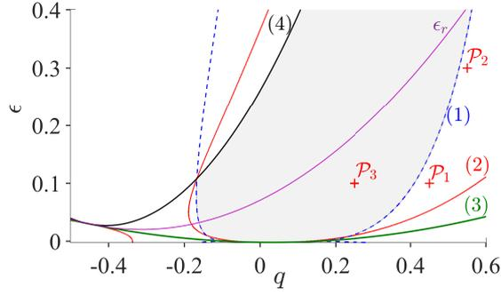
FIGURE 20. Hexagon stability diagram for a shear-thinning fluid with  $\alpha = 10^{-4}$ ,  $Pr = 50$  and  $r = 2.5$ . The curve  $\epsilon_r(q)$  is a boundary above which rolls are stable with respect to homogeneous perturbations. (+) Points where numerical simulations were performed.
