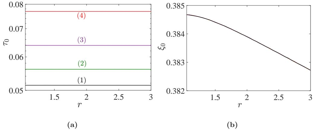
FIGURE 8. Variation of the characteristic time  $\tau_0$  (a) and the coherence length  $\xi_0$  (b) as a function of the viscosities ratio, for different values of Prandtl number. (1)  $\text{Pr} = 50$ ; (2)  $\text{Pr} = 5$ ; (3)  $\text{Pr} = 2$ ; (4)  $\text{Pr} = 1$ .
