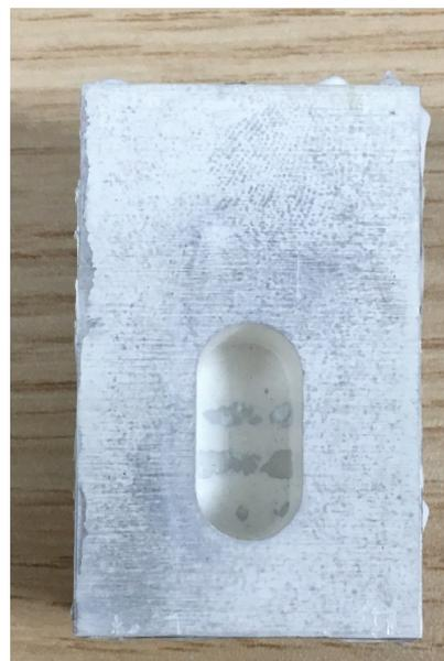
FIG. 10. Picture of the external part of a D<sub>2</sub> type cell containing hydroxide after approximately 6 hours at high temperature.
