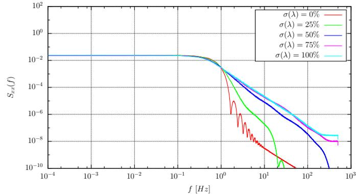
**Figure 7.** Influence of enabling a variation of the turbulent structure sizes (represented by  $\sigma(\lambda)$ ) on the power spectral density with a Gaussian function, a mean  $\boldsymbol{\lambda} = (0.5, 0.5, 0.5)$ , a filling ratio of  $R_f = 2$  and a given turbulence intensity of  $I_\infty$ .
