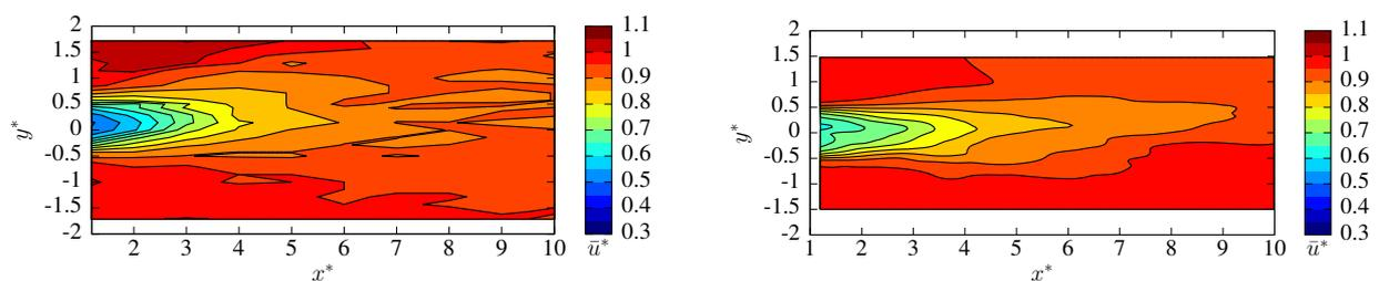
**Figure 9.** Wake velocity comparison with the experimental velocity maps of Mycek *et al.* [22]. Left is the experimental and right is the numerical velocity map for  $\text{TSR} = 3.67$ ,  $I_\infty = 15\%$  and  $\lambda = (0.1, 0.1, 0.1)$ .
