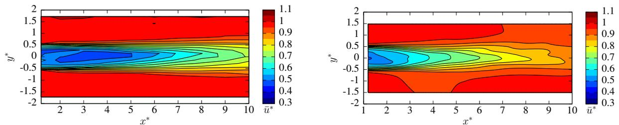
**Figure 8.** Wake velocity comparison with the experimental velocity maps of Mycek *et al.* [22]. Left is the experimental and right is the numerical velocity map for  $\text{TSR} = 3.67$ ,  $I_\infty = 3\%$  and  $\lambda = (0.1, 0.1, 0.1)$ .
