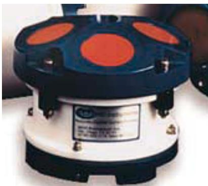
Figure 2: Adcp Workhorse Mariner 600 KHz
