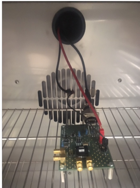
(a) PUF evaluation board inside of the climate chamber
