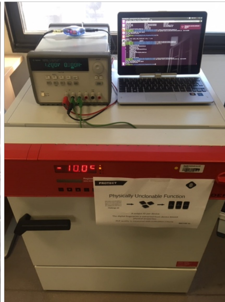
(b) Control of the power supply and the climate chamber
