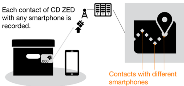
Fig. 2. Asset tracking with zero added energy, zero new signals and zero new equipment in the network
