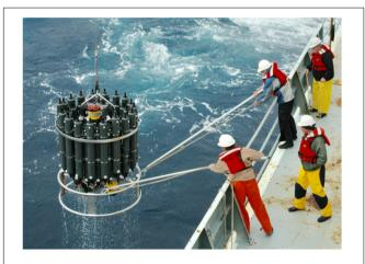
**FIGURE 1** A rosette sampler with Niskin bottles. The conductivity, temperature, depth (CTD) sonde is inside of the ring near the bottom (not visible) (Photo credit: Sabine Mecking, University of Washington).
