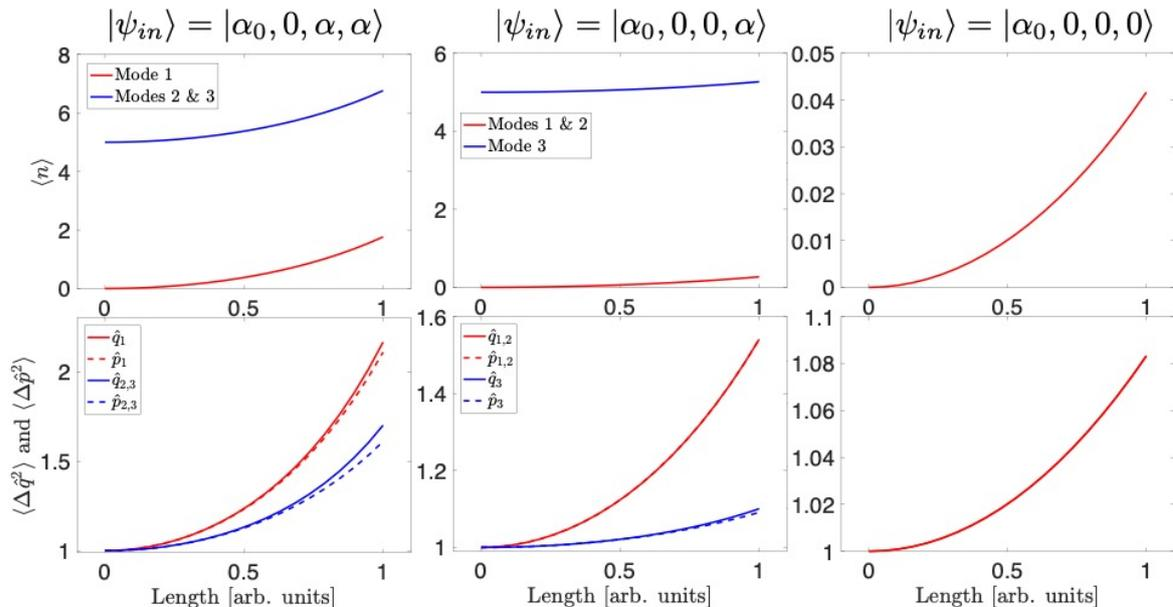
FIG. 9: Top: Evolution of the average photon number of the different modes under TPG. Bottom : Corresponding quadrature variances. For this analysis,  $\kappa = 0.02$ ,  $|\alpha_0|^2 = 100$ , and  $|\alpha|^2 = 5$ .
