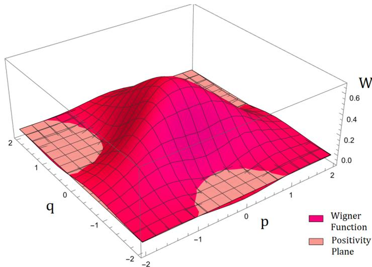
FIG. 16: Wigner Function  $W$  of the state  $|\psi\rangle$  as a function of the canonical quadratures  $q$  and  $p$ . The positivity plane (colored in lighter color) divides the Wigner Function axis between positive and negative values.
