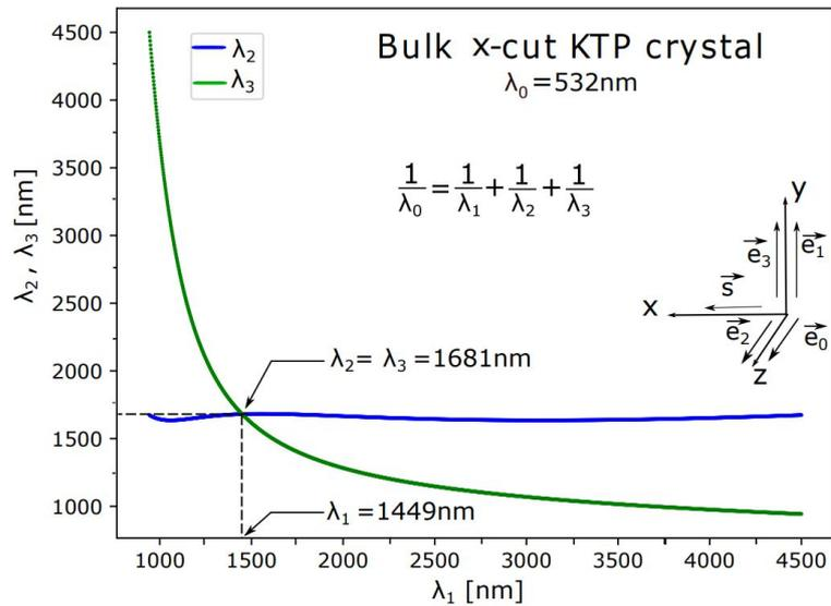
FIG. 2: TPG phase-matching curve in a bulk x-cut KTP crystal pumped at  $\lambda_0 = 532 \text{ nm}$ . The indices  $x$ ,  $y$  and  $z$  stand for the dielectric axes of the crystal, and  $\lambda_1$ ,  $\lambda_2$  and  $\lambda_3$  for the triplet wavelengths.
