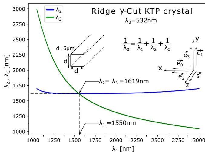
FIG. 3: TPG phase-matching curve in a ridge y-cut KTP crystal pumped at 532 nm with transverse dimension  $d \times d = 6 \times 6 \mu\text{m}^2$ . The indices  $x$ ,  $y$  and  $z$  stand for the dielectric axes of the crystal.
