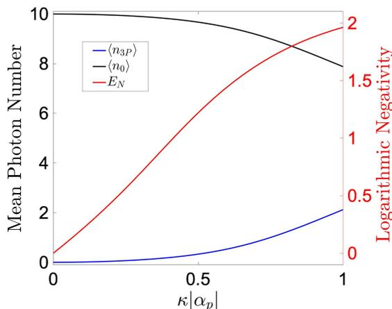
FIG. 13: Red: Logarithmic Negativity of the spontaneous TPG excited by a coherent pump with a mean photon number  $|\alpha_0|^2 = 10$ . Black: Evolution of the pump mean photon number. Blue: Evolution of the mean photon number of the generated triplets.
