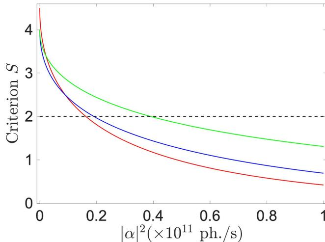
FIG. 12: Evolution of the entanglement criterion  $S$  for different interactions TPG configurations. Red: fully seed TPG with a relative phase of  $\pi/2$ . Blue: double-seed TPG. Green: One mode seeding configuration and  $S$  calculated for the two unseeded modes.  $|\alpha|^2$  is the mean photon number per second of each seeding beam.
