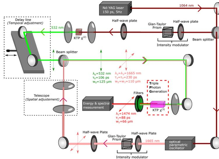
FIG. 7: Experimental setup of a phase-matched TPG in a bulk x-cut KTP crystal pumped at 532 nm and stimulated at  $\lambda_2 = \lambda_3 = 1665$  nm with orthogonal polarizations in the picosecond regime. The dashed lines with double arrows stand for the direction of polarization of the different interacting beams. The values of pulse durations ( $\tau$ ) and waist radius ( $w$ ) are taken at  $1/e^2$ .
