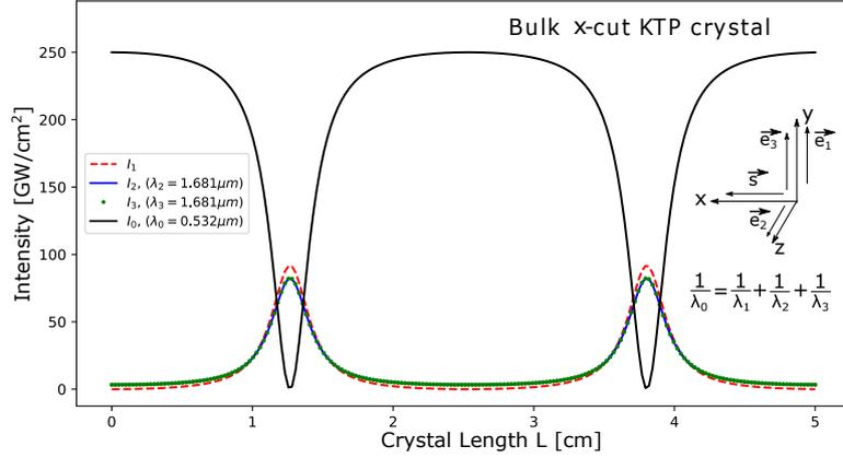
FIG. 5: Intensities of phase-matched TPG, pumped at  $\lambda_0$  and stimulated at  $\lambda_2$  and  $\lambda_3$ , as a function of the crystal length  $L$  of a bulk x-cut KTP crystal pumped at 532 nm.
