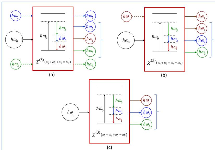
FIG. 1: The three schemes of generation of a 3-photon state at energies  $\hbar\omega_1$ ,  $\hbar\omega_2$  and  $\hbar\omega_3$  in a third-order nonlinear medium pumped at  $\hbar\omega_0$ : (a) stimulation over two modes, at  $\hbar\omega_2$  and  $\hbar\omega_3$  for example; (b) stimulation over one mode, at  $\hbar\omega_1$  for example; (c) no stimulation. The energy levels are described by continuous lines for the matter and a dashed line for the electromagnetic field.
