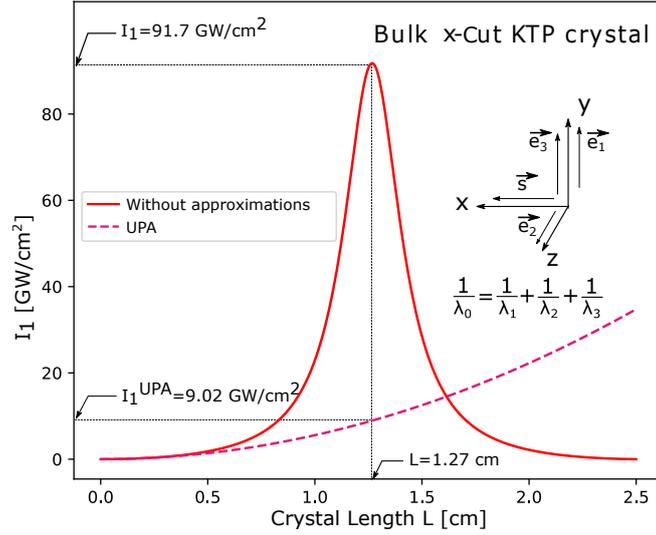
FIG. 6: Intensity generated at  $\lambda_1$  by phase-matched TPG in a bulk x-cut KTP crystal pumped at 532 nm using the general modeling (red curve of Fig. 5) and the undepleted pump and stimulation approximation.
