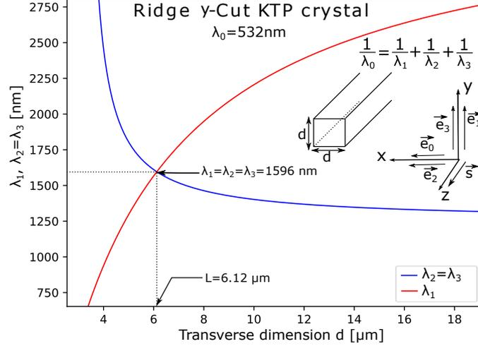
FIG. 4: Partially degenerated ( $\lambda_1 \neq \lambda_2 = \lambda_3$ ) and fully degenerated ( $\lambda_1 = \lambda_2 = \lambda_3$ ) TPG phase-matching curve as a function of the transverse dimension of a ridge y-cut KTP crystal pumped at 532 nm. The indices  $x$ ,  $y$  and  $z$  stand for the dielectric axes of the crystal.
