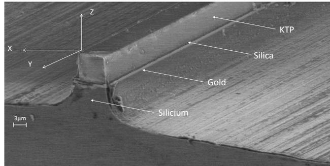
FIG. 8: Electron microscopy image of a KTP ridge waveguide obtained using diamond blade dicing. ( $x, y, z$ ) is the dielectric frame of KTP. The total length along the  $y$ -axis is equal to  $8.6\text{ mm}$ .
