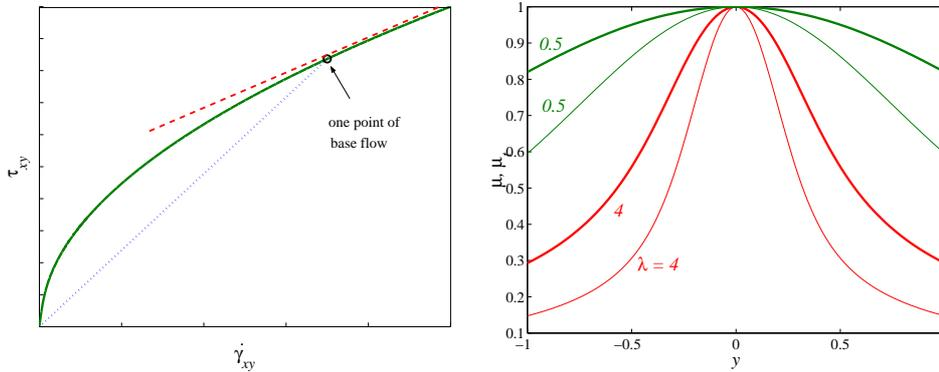
FIGURE 1. Left: Qualitative behavior of  $\tau_{xy}$  versus  $\dot{\gamma}_{xy}$  for a Carreau fluid. The slope of the dotted line is the so-called effective viscosity, the slope of the dashed line is the tangent viscosity. Right: Effective and tangent viscosity as function of the wall-normal coordinate  $y$ , for  $n = 0.5$  and two values of  $\lambda$ . The thick line is the effective viscosity and the thin line is the tangent viscosity
