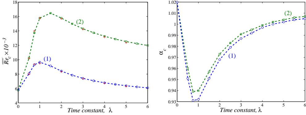
FIGURE 2. Variation of the critical Reynolds number (on the left) and streamwise wave number with the time constant  $\lambda$  at  $n = 0.5$ : the line denoted by (1) (respectively (2)) corresponds to results including (respectively, excluding) the viscosity perturbation. The + signs correspond to unpublished data provided by Chikkadi and Govindarajan (2007).
