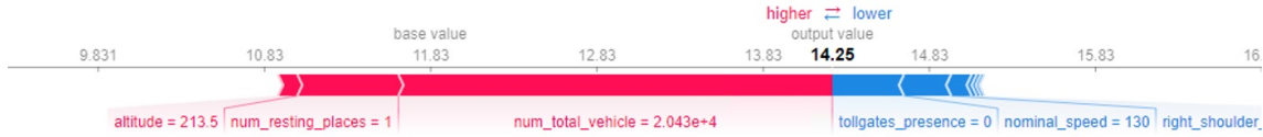
Figure 2: Forceplot of the explanatory variables’ contributions to the estimated crash count for a specific observation. On this example, the traffic has the biggest positive contribution and explains most of the crash count shift from its overall expected value.
